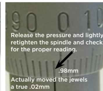
Release the pressure and lightly retighten the spindle and check for the proper reading. .98mm. Actually moved the jewels a true .02mm
