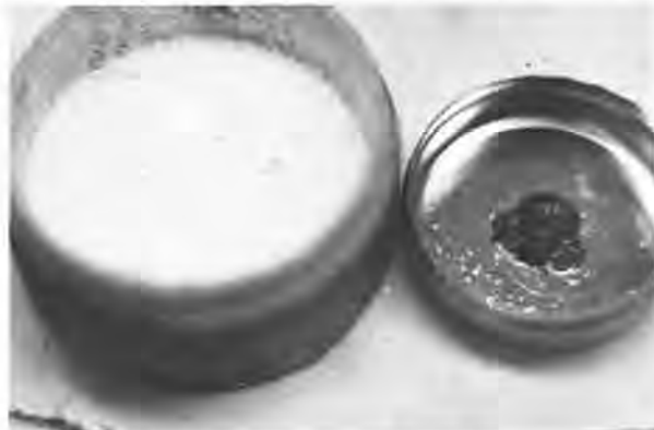
Figure 6. No. 0 oilstone powder and bridle lubricant.
