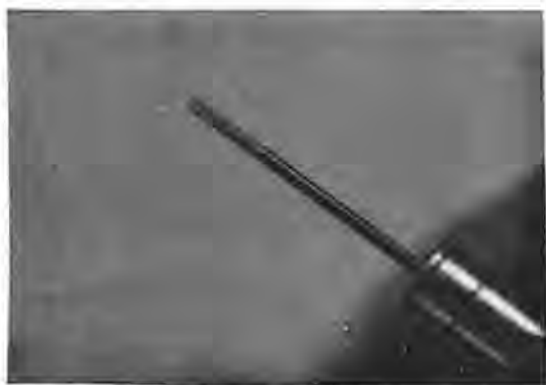
Figure 7. Screwdriver 0.50 mm diameter after being coated with oilstone powder.
