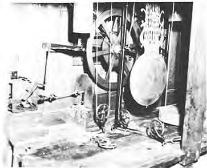
Figure 4. Inside case floor: showing pendulum and calendar gearing; main wheel: 14 1/4 in. diameter.
