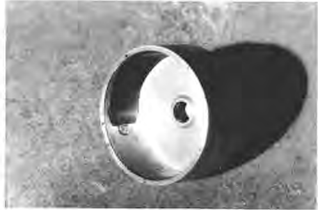
Figure 7. Mainspring brace positioned in barrel.
