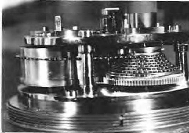
Figure 4. Barrel nearly fully wound.
