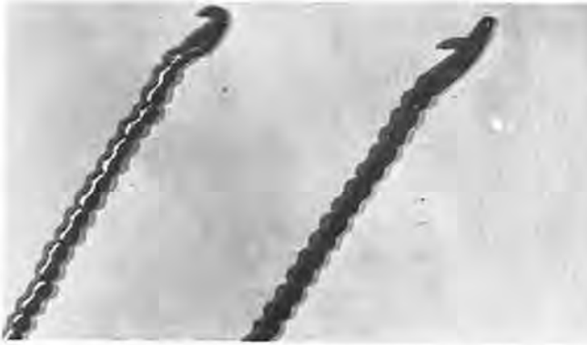
Figure 3. Left—hooks to pin in fusee; right—hooks to pin in hole in barrel.
