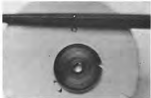
Figure 2. Sealed barrel snap type cap with V notch.
