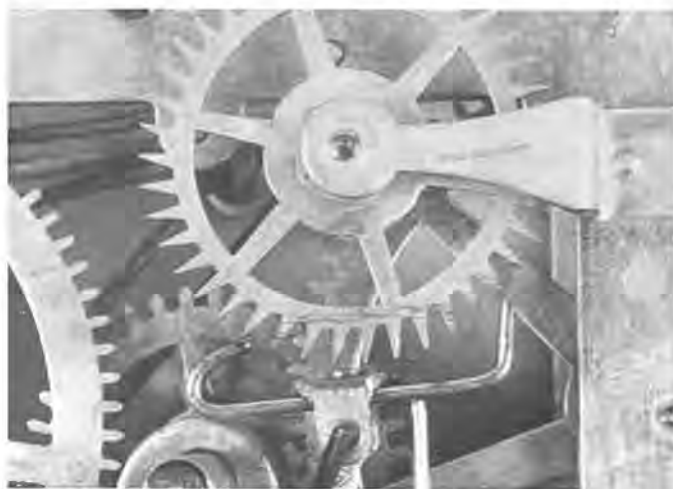
Figure 26. Exit drop and entry lock.
