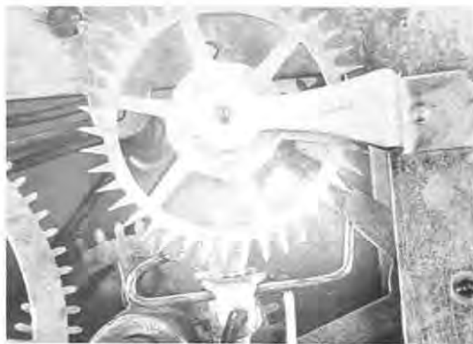
Figure 27. Full recoil of entry pallet.
