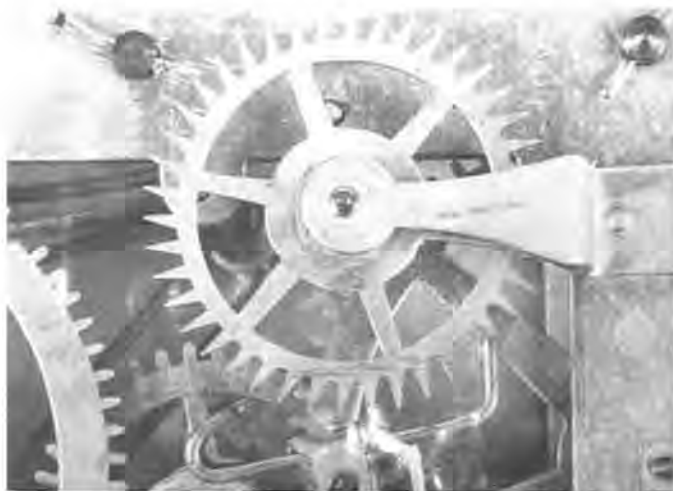
Figure 25. Full recoil of exit pallet.
