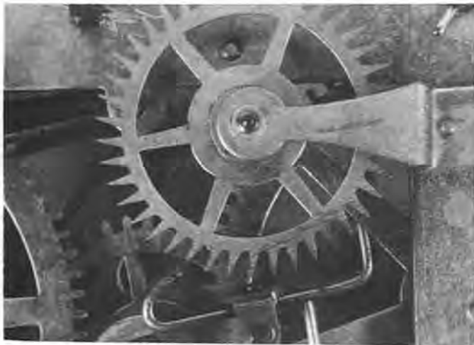
Figure 15. Entry drop following initial adjustment.
