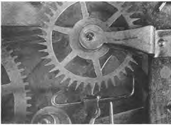
Figure 20. Exit drop following second adjustment.
