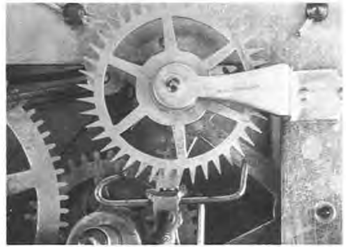
Figure 21. Lack of clearance following second adjustment.
