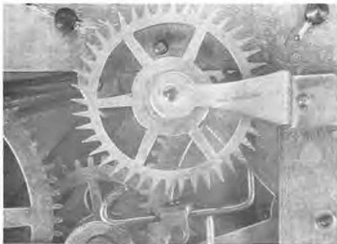
Figure 16. Exit drop following initial adjustment.
