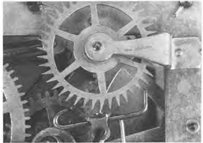
Figure 19. Entry drop following second adjustment.
