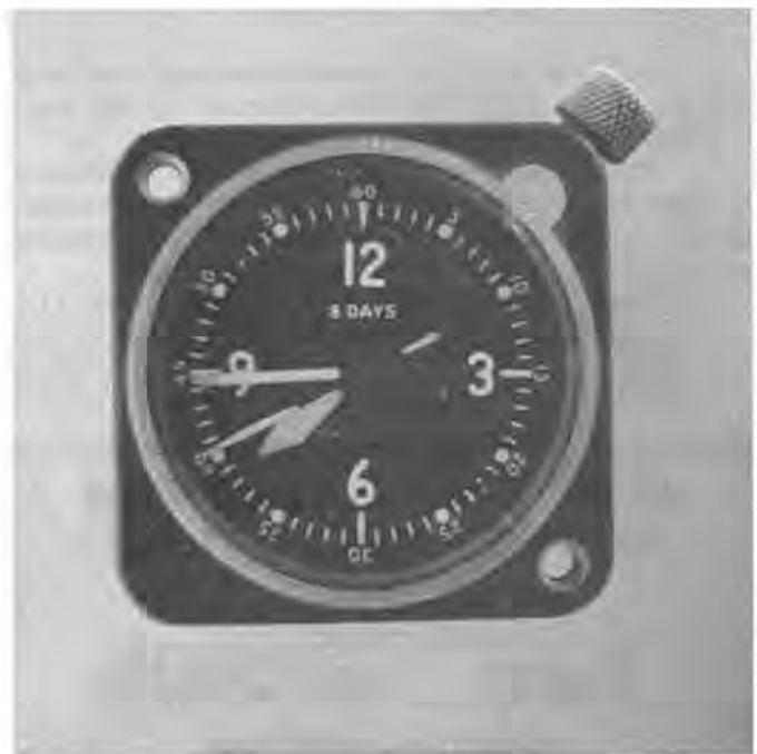
Figure 1. LeCoultre, Model 201, 8-day, 19 ligne, 7-jewel, type A-11 aircraft clock.
