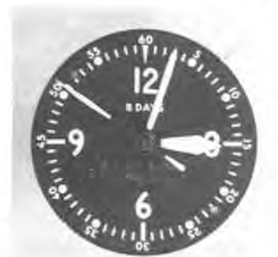
Figure 1. LeCoultre, Model 201, 8-day, 19 ligne, 7-jewel, type A-11 aircraft clock.
