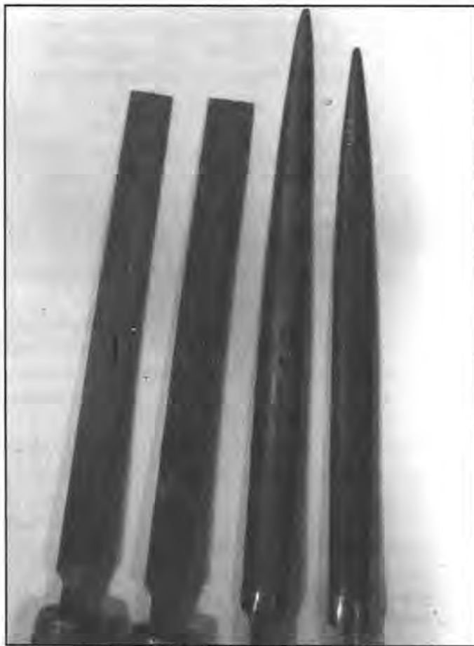
Figure 3. From left to right: (1) pillar, (2) flat, (3) half round fine, (4) half round coarse.
