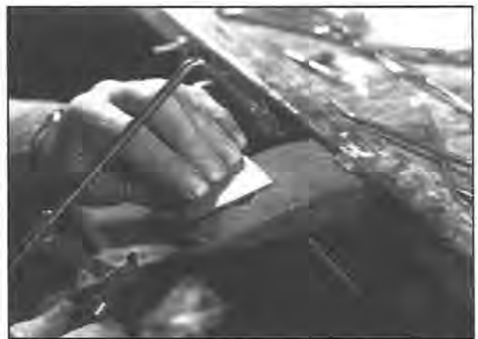
Figure 1. Practice sawing. Note that the saw is being held at about a 30° angle and the bench pin is inverted to allow it to slant downward from the bench, making it easier to saw a straight line.
