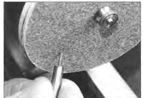
Figure 2. A soft-backed grinding disc sharpens various tools
