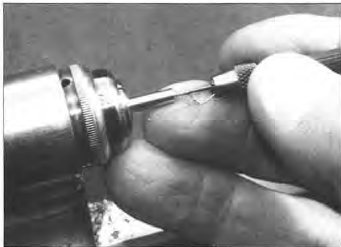
Figure 9. Watch, and clear chips frequently, add lubricant
