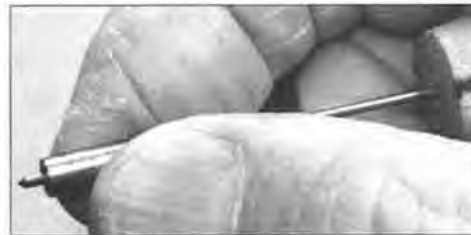
Figure 11. The method of holding "The Magic Center Finder"
