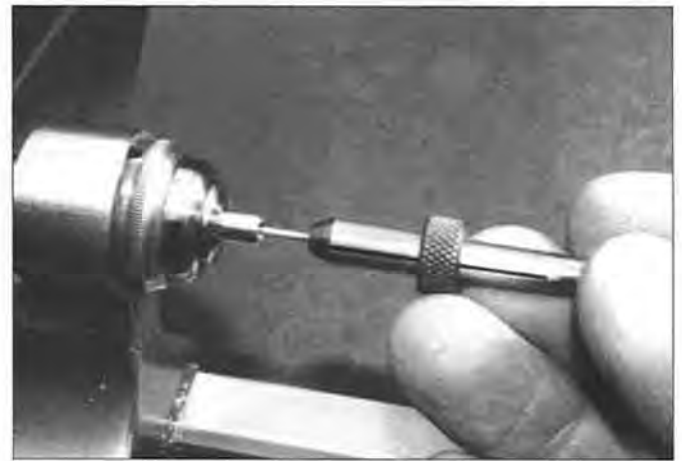
Figure 7. Hold a spade drill lightly so it spins in the event of a hang up
