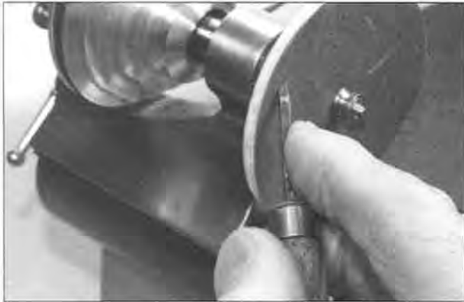
Figure 3. Sharpening a turning graver on a soft-backed grinding disc
