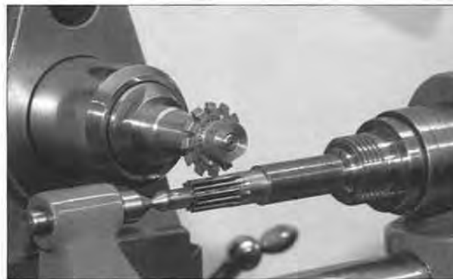
Figure 16. Milling a clock pinion.
