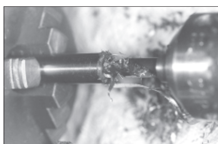
Figure 18. A 19/64-inch (0.2969 inch) drill was used first to a 1" depth.
