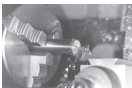
Figure 15. A steel rod was faced flat.
