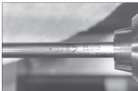
Figure 22. A 0.3115" high-speed steel reamer.
