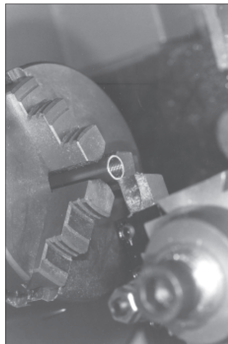
Figure 6. The threaded end was faced flat.
