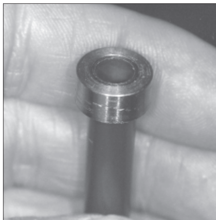
Figure 25. The sleeve pressed on the brake line with a 0.001 interference fit.
