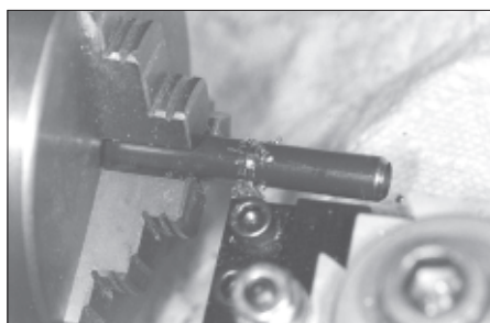
Figure 14. The spindle was parted at the marked length.
