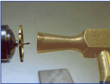
14. The plug was gently tapped fully in place.
