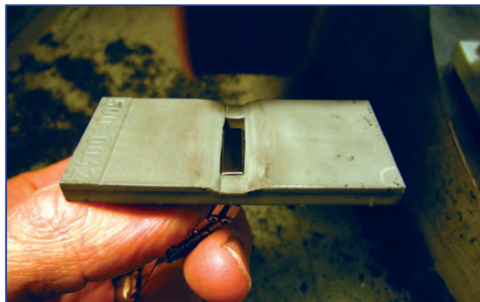
Figure 3: Exposing the satin portions of the bracelet through the hole in the mask to a Bufflex wheel.
