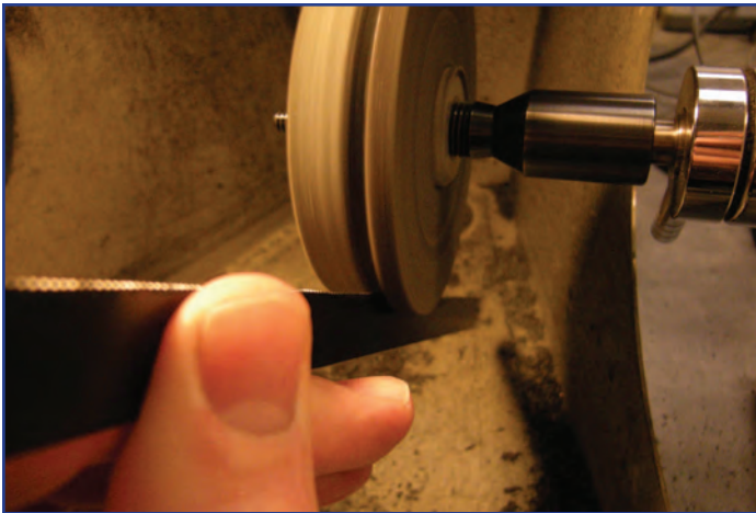
Figure 4: Cutting with a loose hacksaw blade to carve away excess material and leave a raised portion in the wheel.
