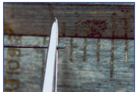
10. The depth of the hole was approximately .5 mm.
