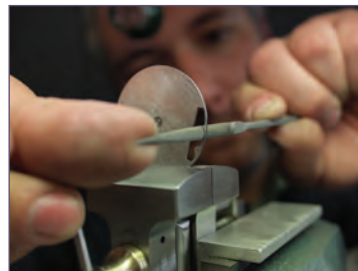
First Intermediate SAWTA Examination 2011: Students hand craft a click spring for a 1910 Lange pocket watch.
