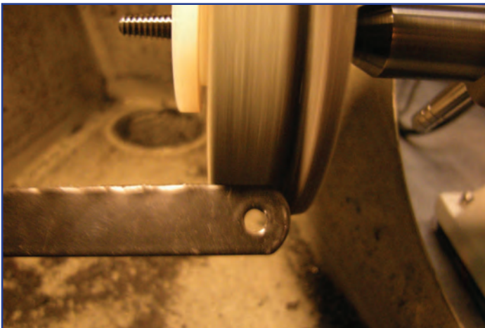
Figure 5: The raised portion is just narrower than the width of the satin sections of the bracelet links.
