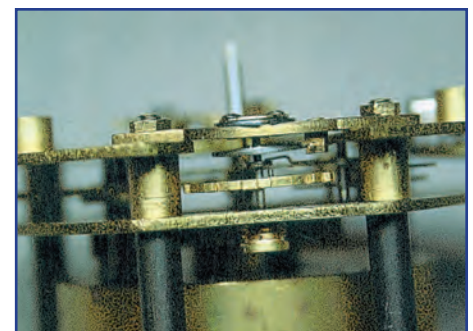
22. Completed pivot repair.
