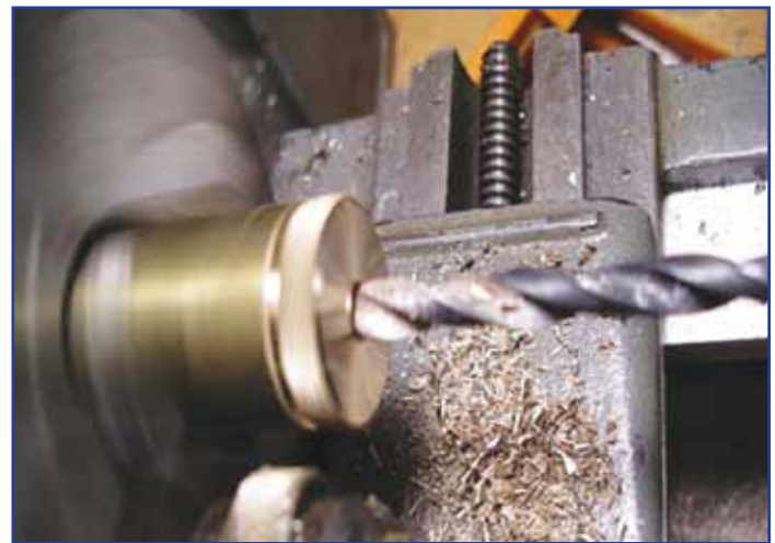
Figure 14: The lock nut is drilled for a 75% thread depth.
