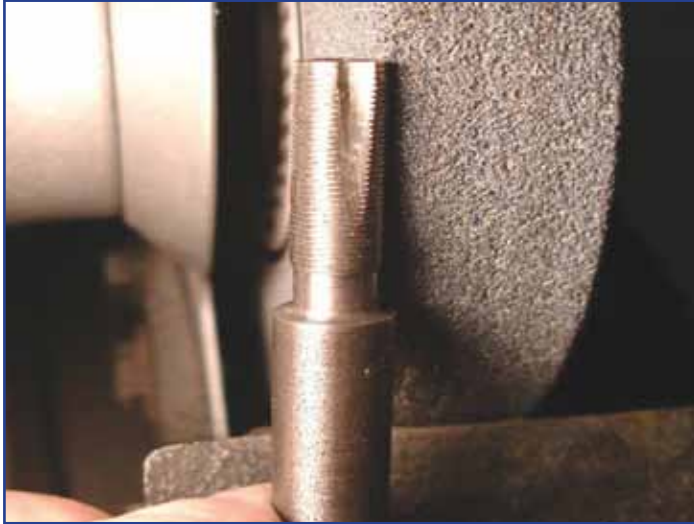
Figure 11: Using a coarse grinding wheel.
