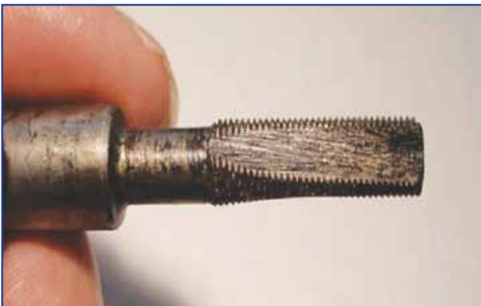
Figure 12: The finished tap.
