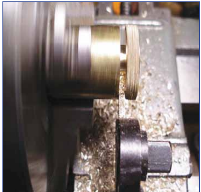
Figure 18: Lock nut parted from the stock with cut-off tool.
