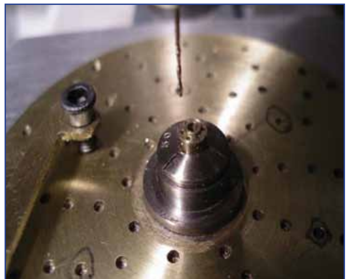
Figure 2: Drilling the lantern pinion.
