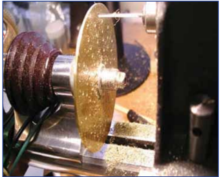
Figure 5: Using the lathe milling attachment to drill the index plate.
