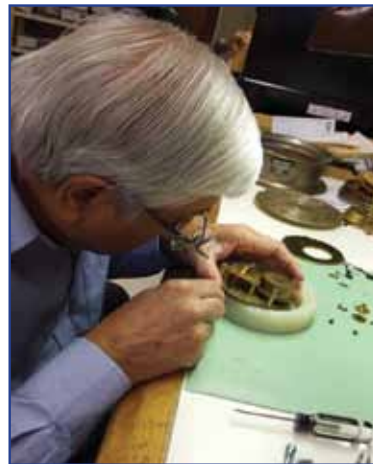
Chelsea Clock master clockmaker Bupat Patel examines the Ship's Bell Clock escapement mechanism, which is still manufactured and hand-assembled the same way today as it was when this timepiece was originally made in 1918.
