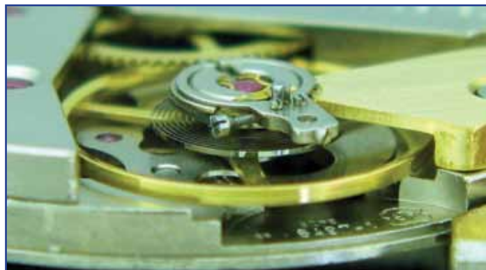
Figure 6: The assembled 6497 oscillator.
