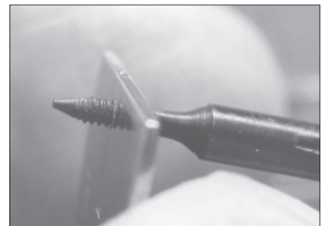
Figure 6. The number one tap corresponds to the #1 thread die in the screw plate.
