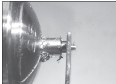
Figure 19. A relief cut was made at the head to allow the stud to seat properly
