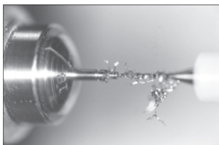
Figure 35. Stainless steel wire was turned to shape and drilled.
