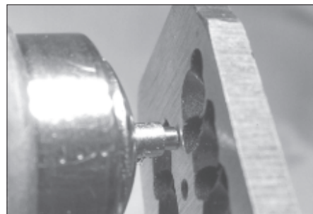
Figure 14. The shoulder was turned down to fit properly in the clearance hole.
