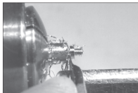
Figure 20. The threaded stud was parted.
