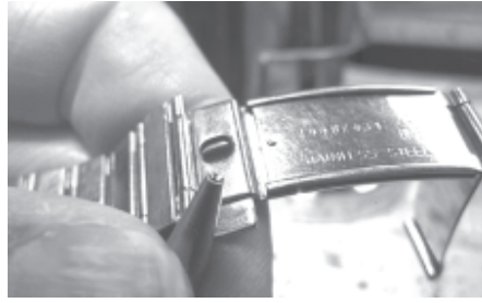
Figure 29. A conical stake was used to chamfer the sharp edge.
