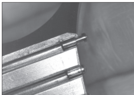
Figure 37. The new end cap was turned down to a tight press fit in the case lug tube.
