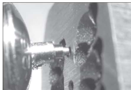
Figure 13. The shoulder was tested for fit in the center clearance hole of the screw plate
