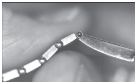
Figure 34. The end cap was missing.
