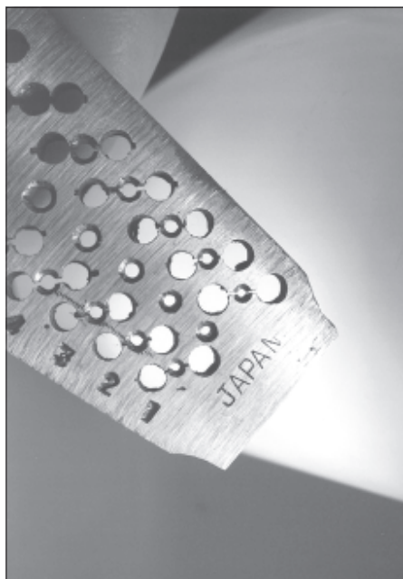
Figure 7. The dies in the screw plate are numbered in whole millimeters. The center hole between each die determines the proper diameter prior to threading.
