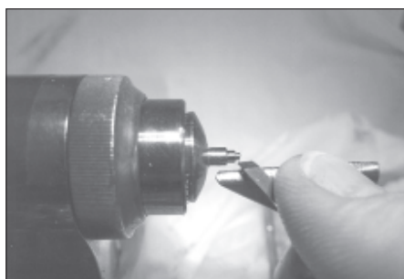
Figure 12. A shoulder was turned down to the correct diameter for threading.
