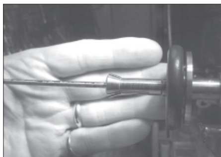
Figure 9. The opposite end of the lathe spindle was threaded with a .275 x 40 tap. A collet that fit the antenna was threaded into the spindle to prevent any whipping action.
