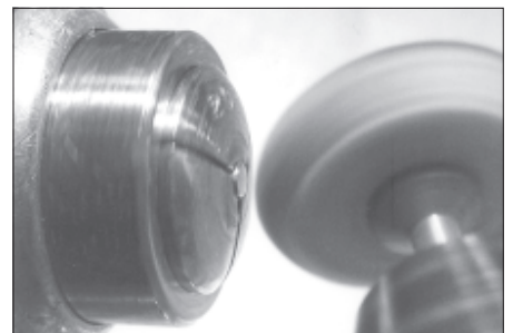
Figure 24. A hard fiber disc charged with compound imparted a fine polish.
