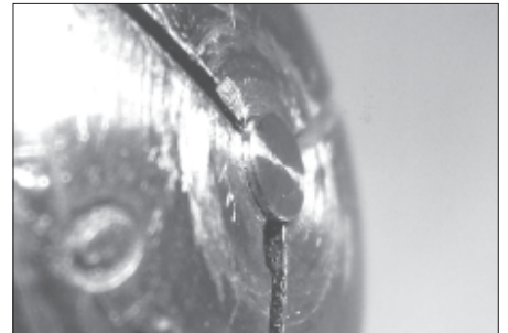
Figure 23. The stud was reversed, held by its head and slightly ground to remove tool marks.
