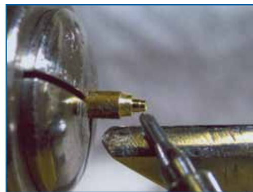
Figure 3: A brass mandrel was turned to fit the hour wheel.
