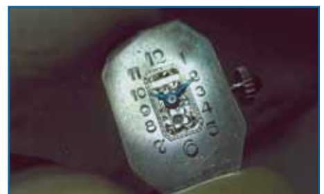
Figure 9: The new hands in place.
