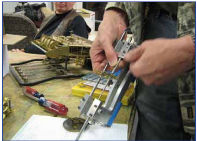
Richard Zielike setting up a two wheel and pinion in a depthing tool to locate correct pivot hole locations.
