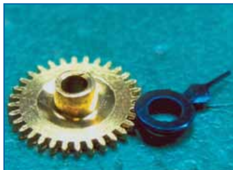
Figure 2: The hour wheel with a robust hand post and the new hand with a tube that is too small.
