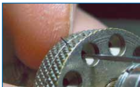
Figure 8: A five-sided taper broach was used to enlarge the minute-hand hole.
