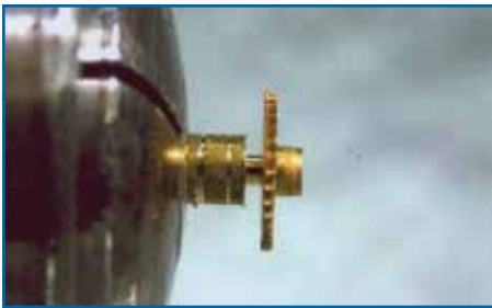
Figure 4: The hour wheel was pressed tightly onto the mandrel.
