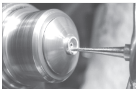
Figure 9. Very fine cuts were taken to remove the internal serrations.
