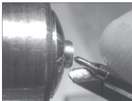
Figure 20. The sleeve was slightly longer and was turned flush with the cap.
