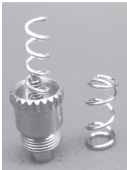
Figure 30. The relative positioning of the new spring and screw
