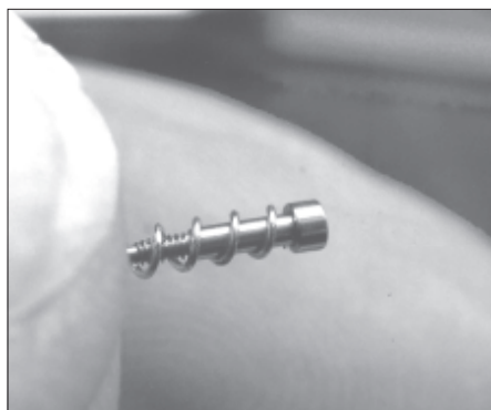
Figure 29. The push screw inside the spring
