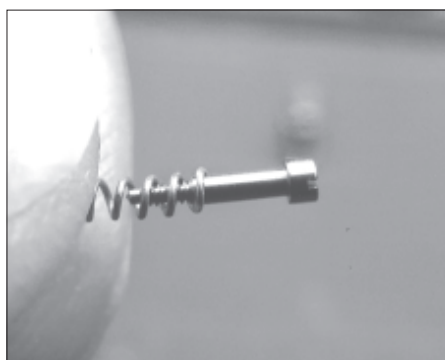
Figure 26. The spring inside diameter was too small.
