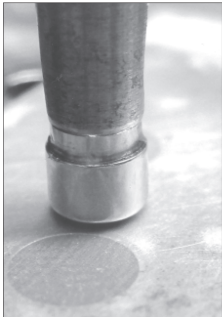
Figure 18. Red threadlocker was applied to the sleeve as it was pressed in place.
