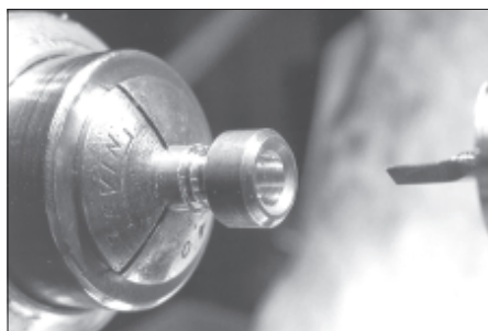
Figure 12. The bushing was pressed onto the mandrel.
