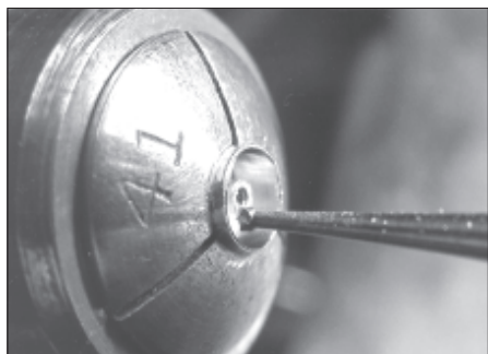
Figure 10. A fine cut finish was created inside the cap.
