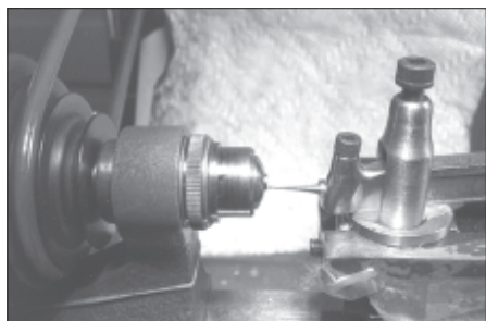
Figure 7. The burr was held in a table rest.
