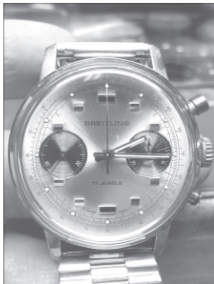
Figure 1. A Breitling vintage chronograph missing a push button cap and spring
