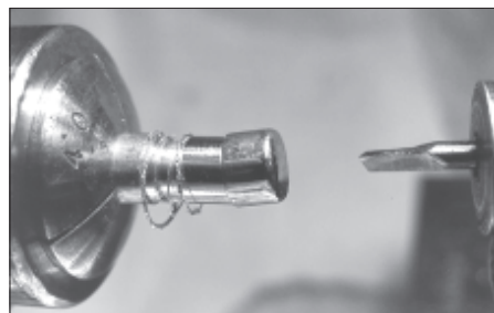
Figure 14. The sleeve was tested for fit in the cap.
