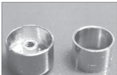
Figure 17. A view showing the substantial thickness of both the cap and sleeve.
