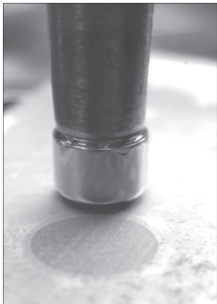
Figure 19. The sleeve was fully pressed into the cap.
