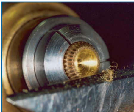
Figure 1. The new crown was bored out
