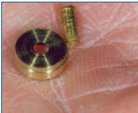
Figure 4. The post separated from the crown as the crown was being faced flat
