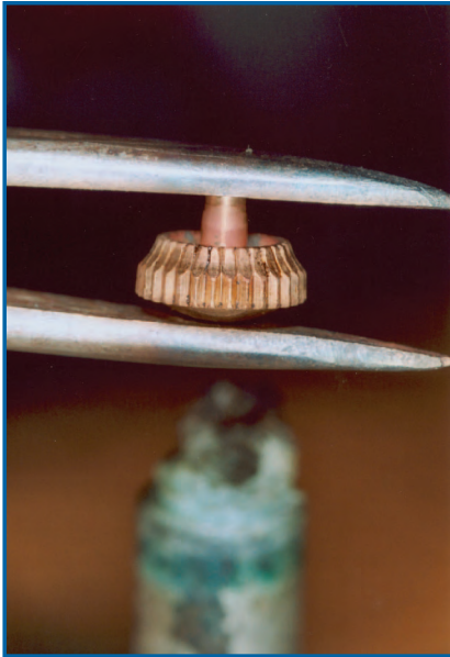
Figure 7. The new post was soft soldered in place
