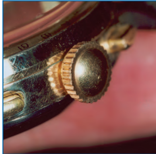
Figure 8. The new crown installed
