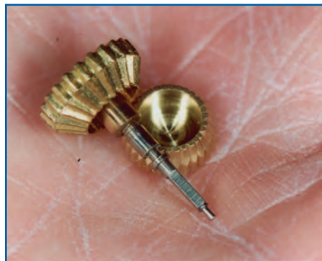
Figure 5. A pocket watch crown was found with the proper threaded post
