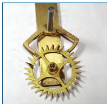
Figure 2: Jig drilled with 2 holes 0.125" diameter at required center distance.
