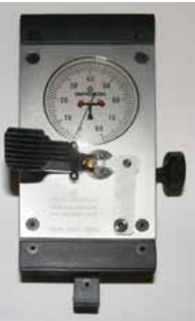
Figure 1: Bergeon escapement tester (Ref. 2229-03).
