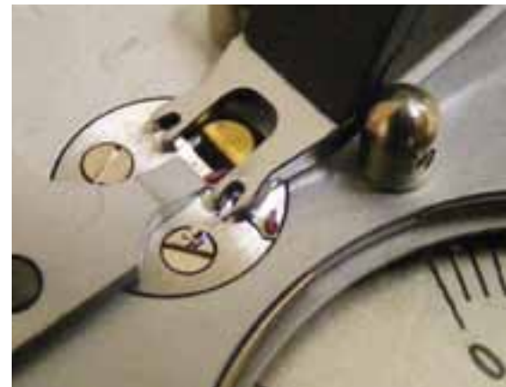
Figure 3: The pallet stone adjustment.
