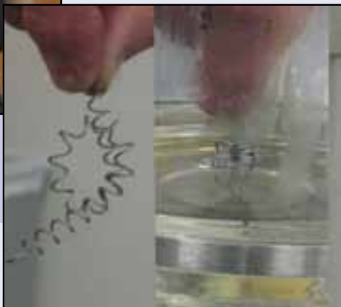
Stunning example of memory returning to its original shape when heated in hot water.
