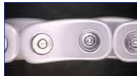
Figure 4: End with cap (remove pin by pushing on center of this side).
