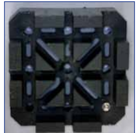
Figure 3: Bergeon 6744 - Support for Bracelet Sizing Tool.
