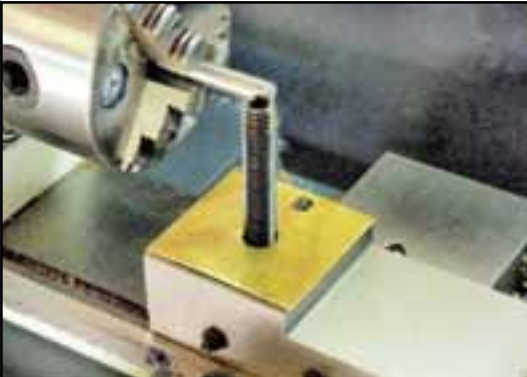
Figure 01.04 The 7 x 12 lathe with a modification to the tool post height.
