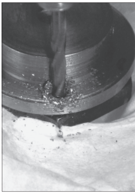
Figure 19. The #43 drill was used to drill through the flange only, providing clearance for the 2-56 screws.
