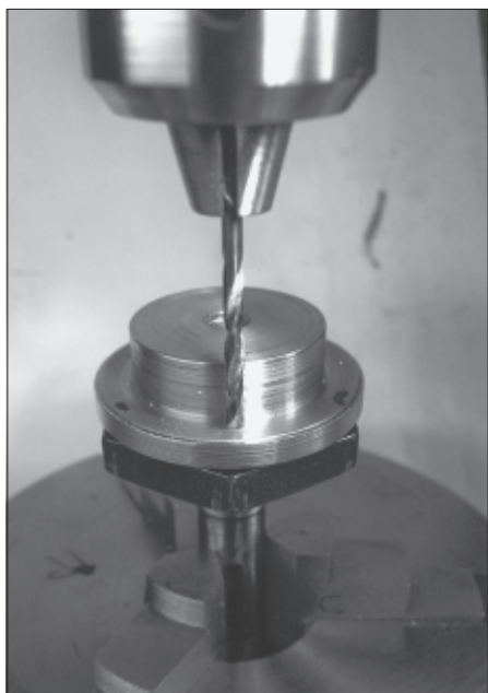
Figure 17. The y table was moved back until the drill was positioned over the flange.
