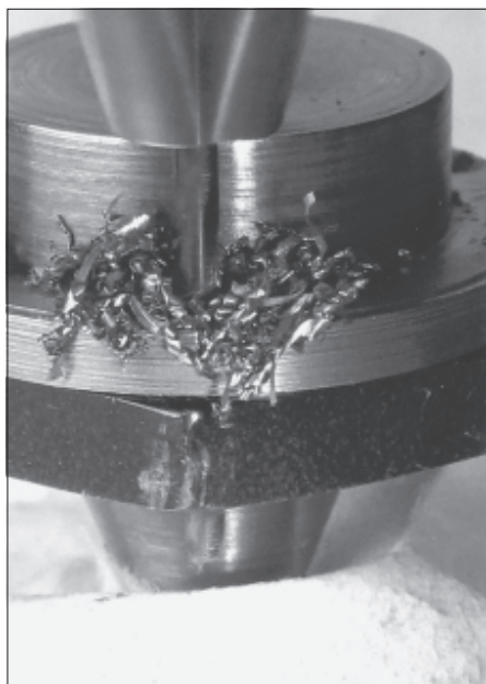
Figure 18. The #50 drill was used to drill through both the flange and the hex.
