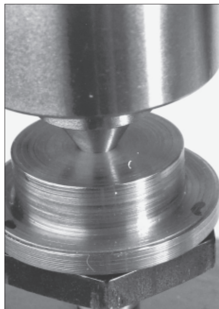
Figure 14. The x-y table was adjusted until the center located the hole in the workpiece.
