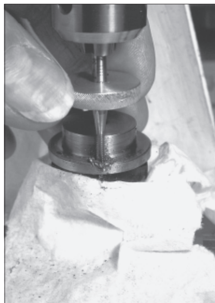
Figure 20. The knurled aluminum disk provided a delicate feel while threading the hex. The tap turned freely in the mill chuck, which maintained a vertical axis.
