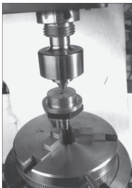
Figure 13. A live center was placed in the mill head and used as an aid to center the workpiece.
