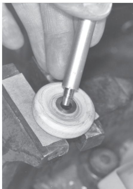
Figure 52. A mandrel was made out of aluminum.
