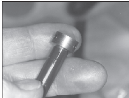
Figure 43. The sleeve affixed onto the spindle.
