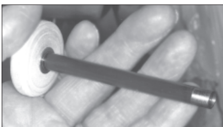
Figure 59. A completed spindle
