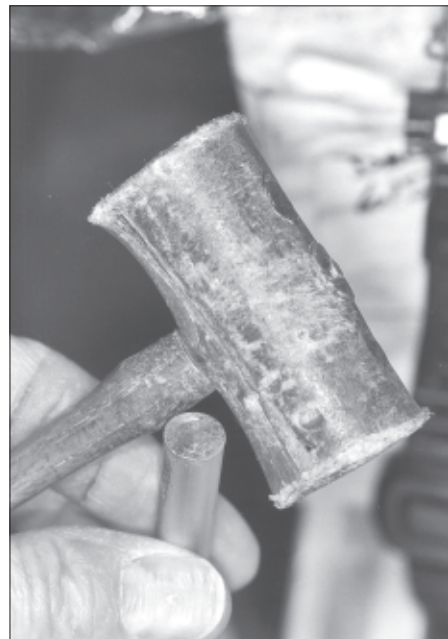
Figure 53. A rawhide hammer and the mandrel were used to drive the sleeve into the wheel.
