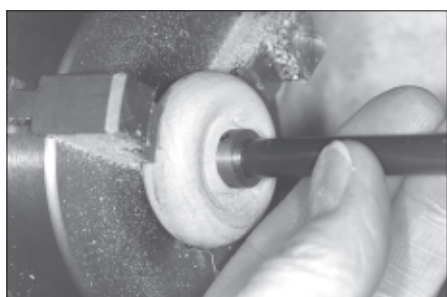
Figure 50. Before removing the wheel from the lathe, the sleeve was tested for fit.
