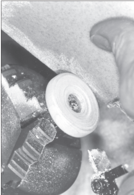
Figure 57. The wooden grip was then sanded smooth.
