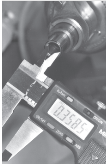
Figure 60. The bore of the Levin® lathe was larger at the grip end.
