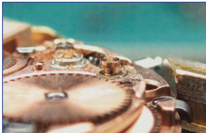
Figure 2: A view showing the extent of the wear on the post.
