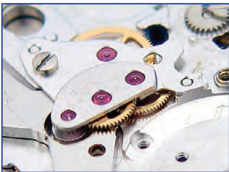
View of stator, rotor, and gear train with bridge installed.
