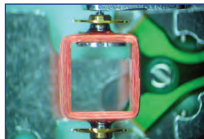
Above: View of the mobile frame wrapped in wire to form the coil with pivots at either end, which rotate within jeweled bearings.
