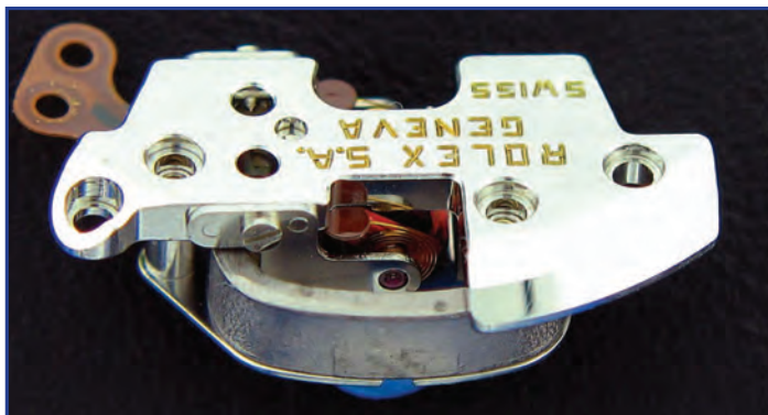
Enlarged view of the motor complete. While the motor can be completely disassembled and serviced, the parts are not available separately. The motor is only available as a complete unit from Rolex.
