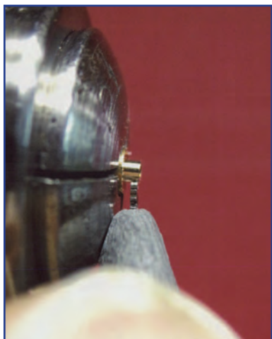
Figure 7: The wheel was used to gage the thickness of the repair piece.
