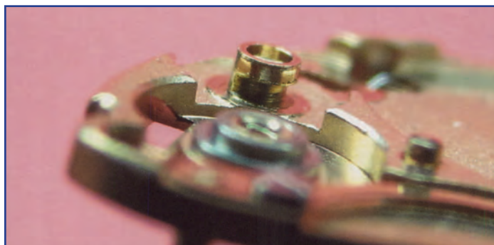
Figure 3: The depth of the wear nearly reached the internal threads.
