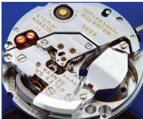
When out of the case the movement definitely has a robust look with an overall diameter of 29.75 mm and a height of 6.35 mm (7.11 mm for the 5055).
