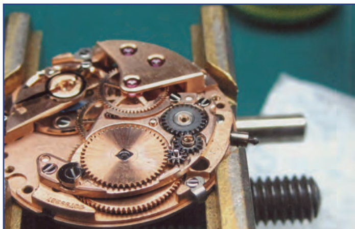
Figure 1: The winding gear arrangement was exposed after its cover plate was removed.
