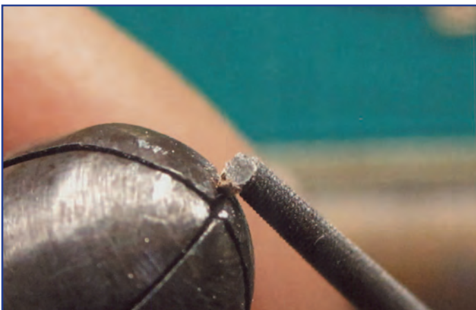
Figure 12: The inside contour was filed to conform to the groove.
