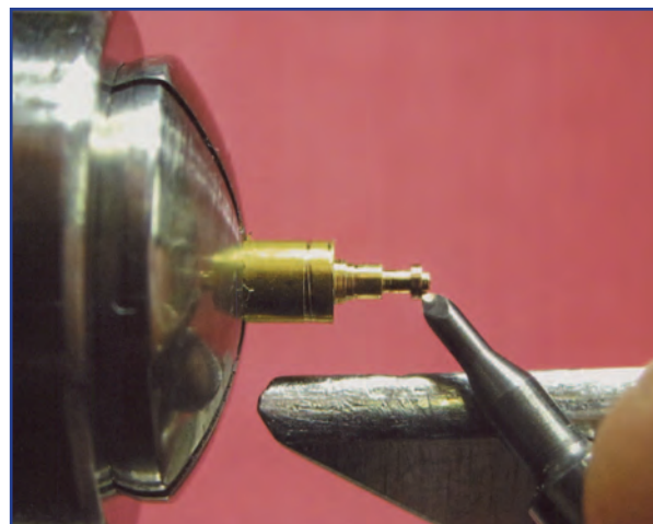
Figure 9: A mandrel was made to a tight fit inside the bushing.
