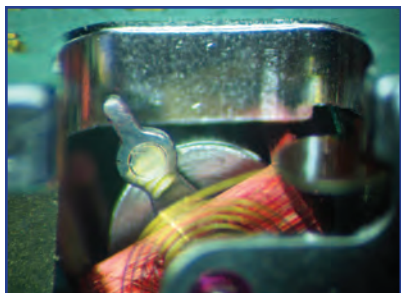
View of the finger attached to the mobile frame. It interacts with the pallet to convert the movement of the mobile frame to the mechanical motion that ultimately drives the hands of the 5035. Note the small circular magnet.
