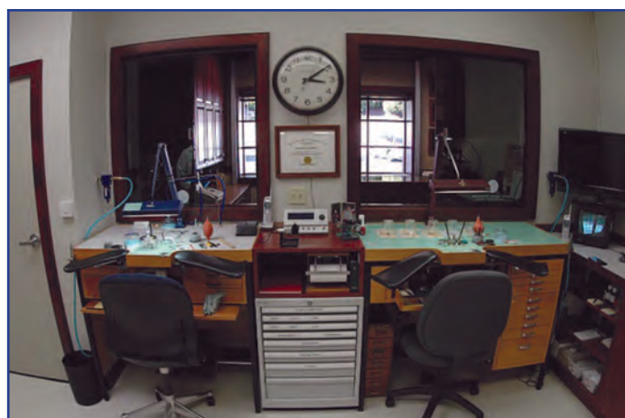
Figure 5: Workbenches divided by Lista parts cabinets to keep frequently-used materials within reach.
