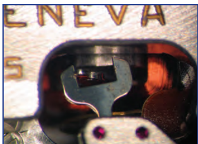
View showing the pallet and finger in one extreme position before impulse.
