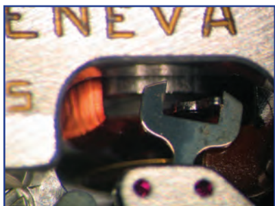
View showing pallet and finger after impulse in the other extreme position.
