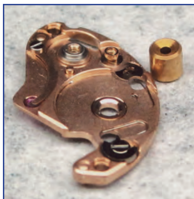
Figure 4: A bronze clock bushing was used.
