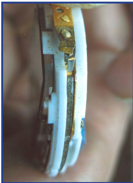
Figure 10. View of repaired contact spring installed.
