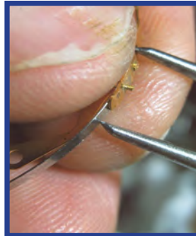
Figure 7. After second hole drilled, springs again riveted. Divider used to scribe proper length on mainspring.
