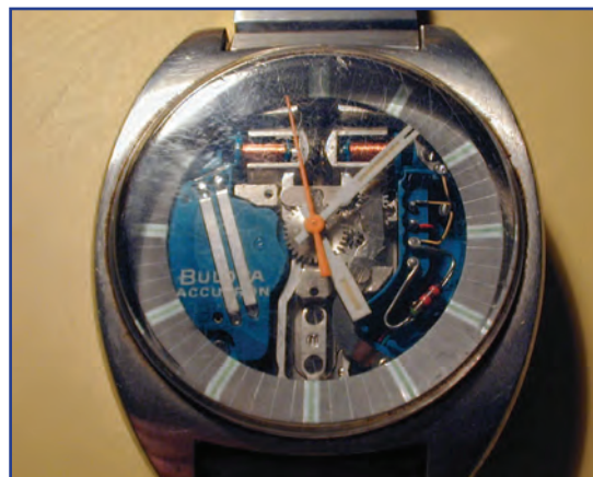
Tuning fork integrated in the Bulova Accutron
