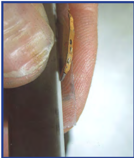
Figure 9. Spring tip polished on ceramic slip.
