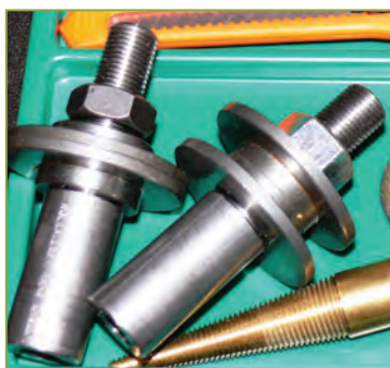
Specialized con-loc arbors utilized with Artifex wheels.
