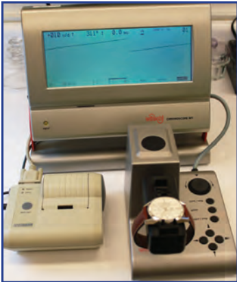
Equipment to measure the accuracy, amplitude and beat of mechanical watches.
