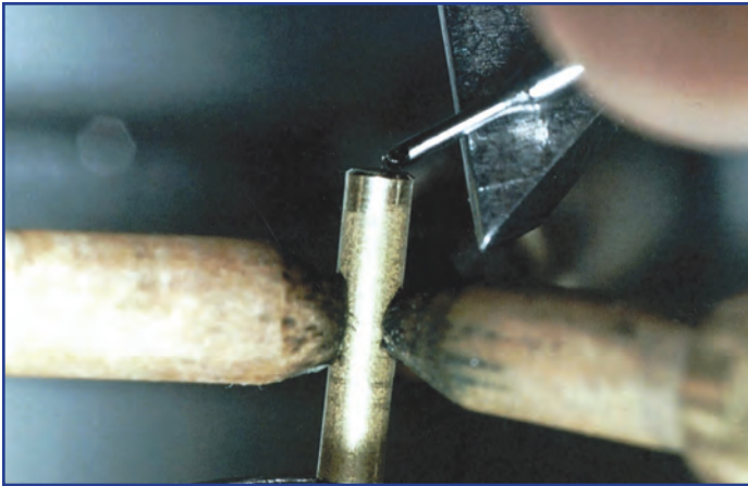
Figure 8: The cone can be turned with a graver.
