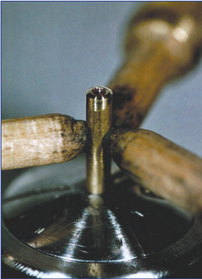
Figure 4: A steady rest holding the protruding needle.
