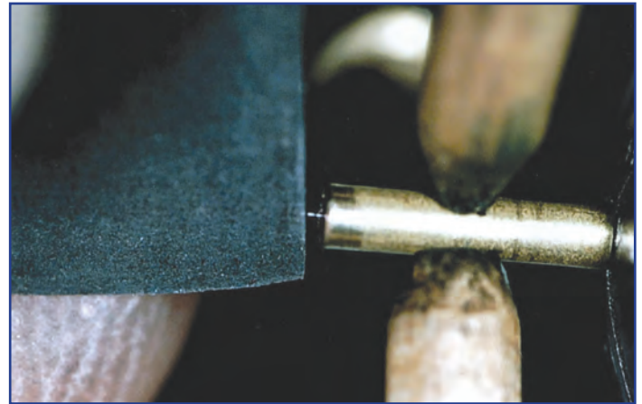
Figure 6: A diamond slip grinding the pivot into shape.
