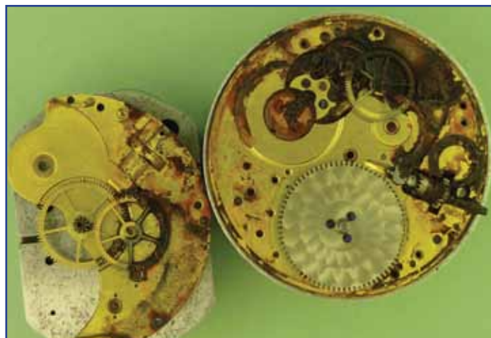
Figure 5: Removing the train bridge showed all train wheels were rusted.
