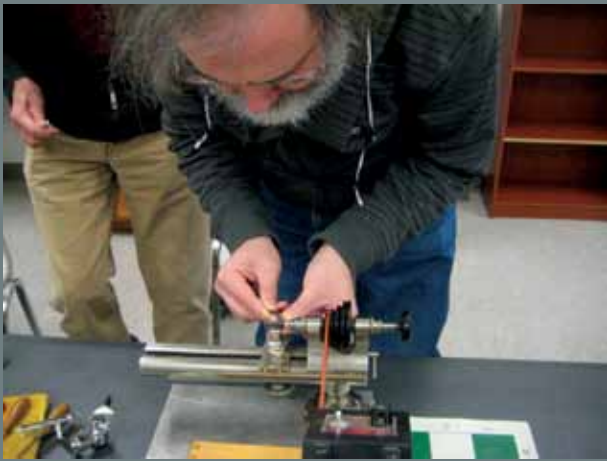
Jeff Pomeroy practicing graver turning of soft brass on a jeweler's lathe.
