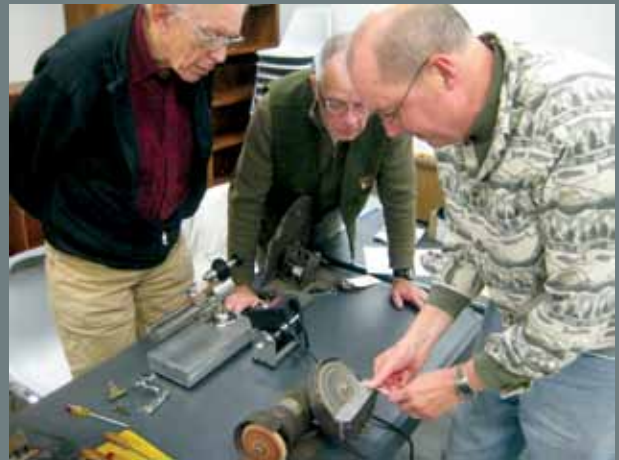
Richard Zielike demonstrating graver sharpening on a slow-speed angle grinder with adjustable table.
