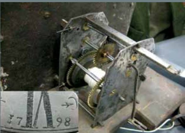
1798 date engraved on front of dial and the short train movement for driving only the hour hand.
