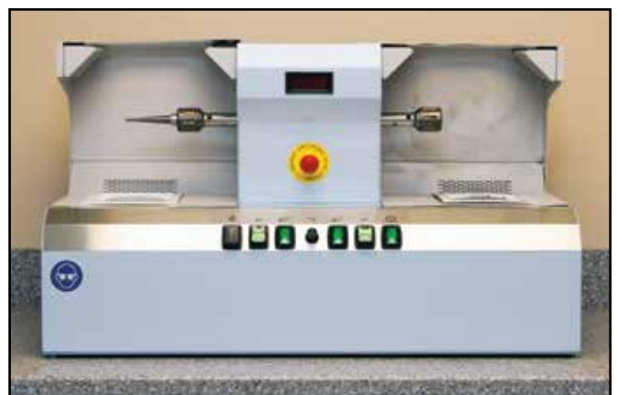
The polishing machine, PM2, was purchased through Rolex. It has variable speed, suction fans, LED lighting, and a collet-style chuck system for ease in changing out mandrels.
