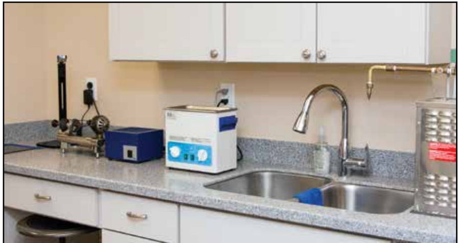
Polishing room. Left to right: The lathe for turning cases, bezels, and backs during refinishing, as well as making odd parts and tools as necessary. A heated drier for drying cases, bracelets, etc., during cleaning and refinishing. The heated ultrasonic, which is used mainly for cleaning watch components regardless of whether or not a refinish is in progress. Some quick service jobs need to be cleaned or steamed, or as requested by customers. The boiler steamer is to the right of the sink. It is excellent for forcefully removing contaminants from watch cases and bracelets.
