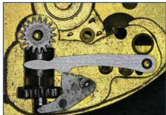
Figure 24. Testing the yoke in hand-setting position.
