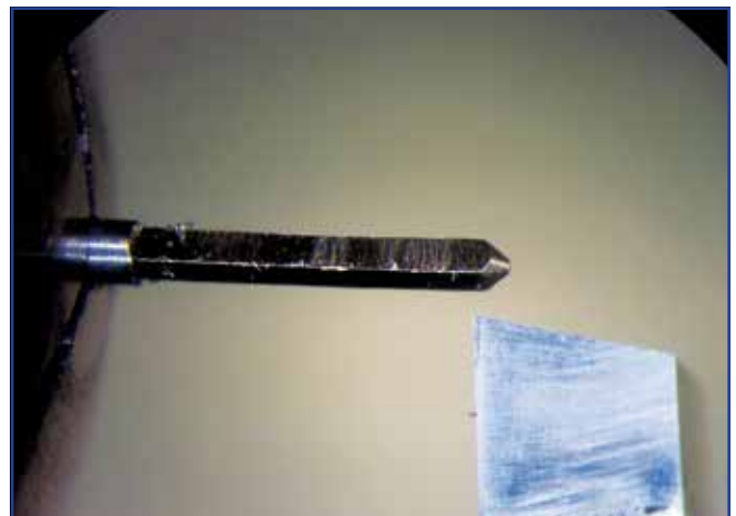
Figure 3. Square broach for sliding pinion milled in the lathe.
