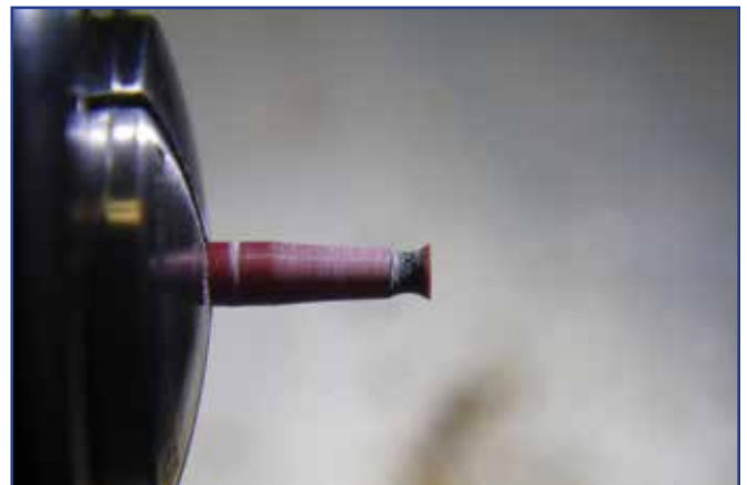
Figure 10. Degussit stone after shaping it with various diamond files in the lathe.
