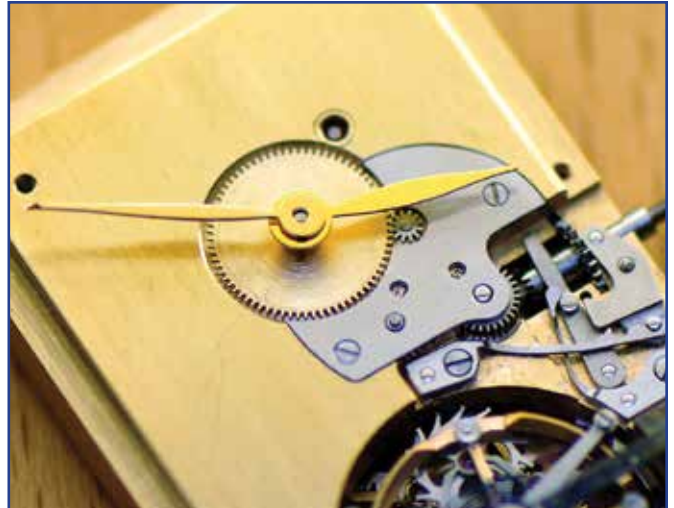
Figure 18. Motion work, winding and setting parts assembled together for testing.
