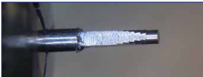
Figure 4. Square broach for sliding pinion after turning incremental steps and a cylindrical pilot.
