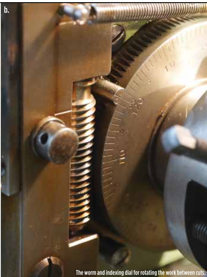
The indexing handle and dial, which allows one to change the orientation of the pattern bar between cuts.
