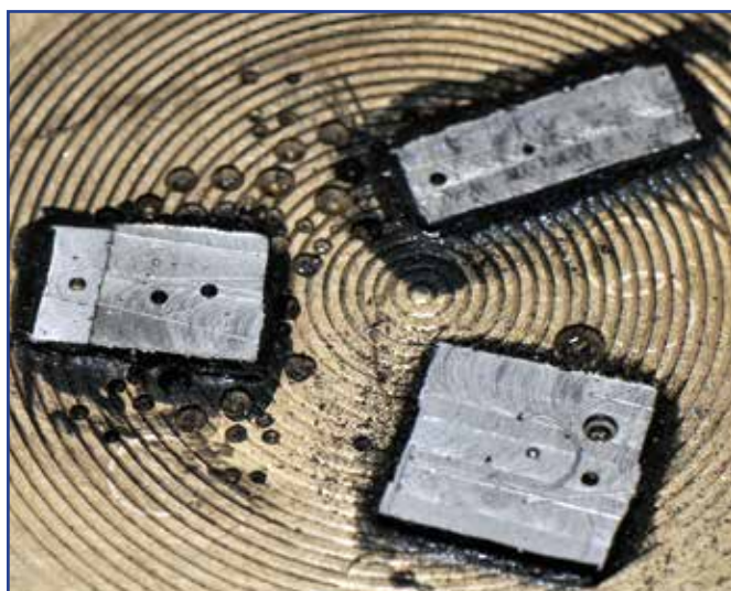
Figure 13. Yoke, yoke spring, and setting lever, drilled and scribed to shape.
