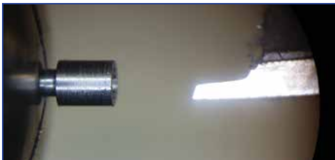
Figure 5. Sliding pinion being bored out in the lathe.
