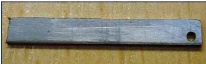
Figure 23. Prepared piece of steel for grinding and filing the yoke.
