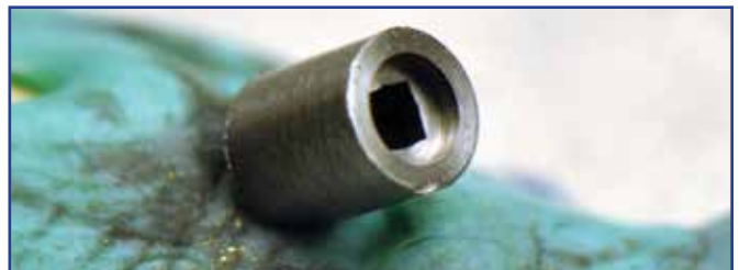
Figure 6. Sliding pinion with its square hole and bored recess for leaves.
