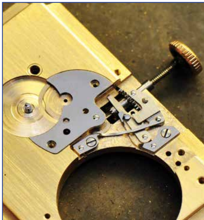
Figure 14. Winding and setting parts after milling and filing the final shapes, with the motion work mainplate area prepared with posts, maintaining bridge, and recesses.
