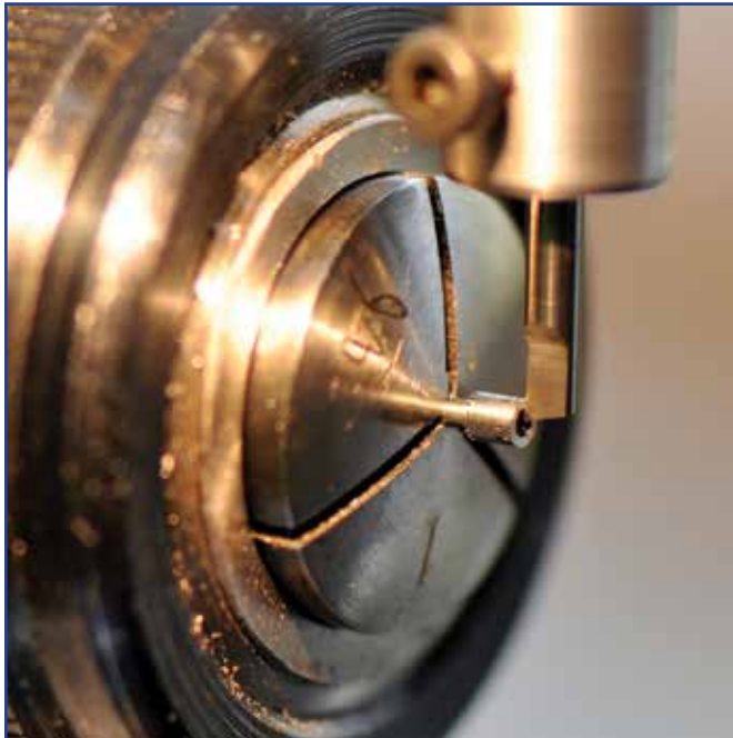
Figure 8. Setting up the broach on the center of the sliding pinion in the F1.
