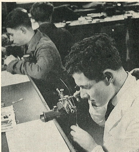
"Pivoting" is a delicate job for the second year students in Swiss horological schools. These eighteen-year-old boys, whose fathers and grandfathers were watchmakers, are learning the skill of polishing and adjusting pivots to the finest tolerances.
