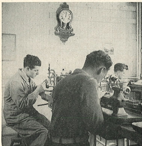
Third-year students in the public-sponsored watch-making school at Le Locle, Switzerland, learn how to grind and polish the parts for the watches they must complete for graduation. They are pictured turning countersinks and adjusting fittings. In the background is a Neuchatel clock which the Swiss made famous between 1760 and 1820.
