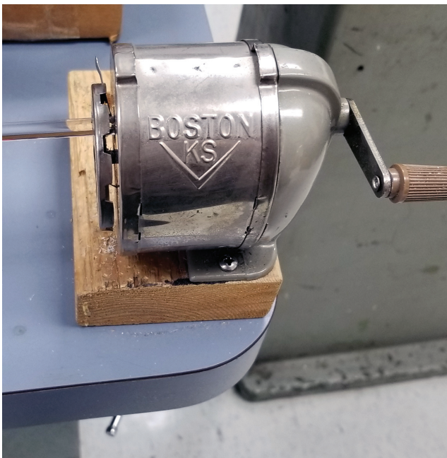
Fig. 2. An old-fashioned hand-turned pencil sharpener can be used to sharpen plexi sticks.
