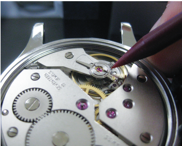
Fig. 6. Use a plexi stick to adjust beat error.
