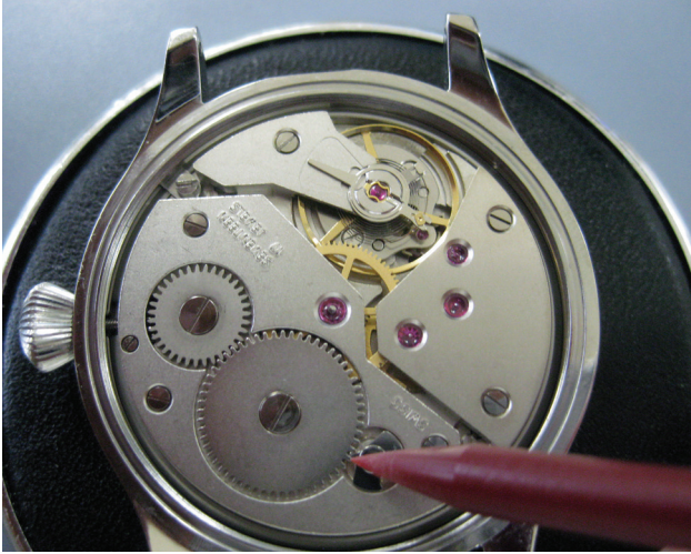
Fig. 4. Blocking the ratchet wheel.
