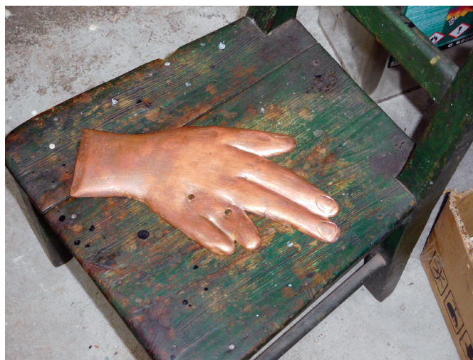
Where a clock hand is really a hand. This indicates the time on the 24-hour dial. The hand is copper and is awaiting gilding with gold leaf.
