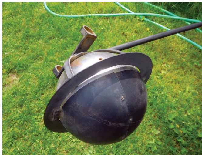
The moon changes phase as the dial rotates. A slider keeps the moon positioned in the ecliptic circle.
