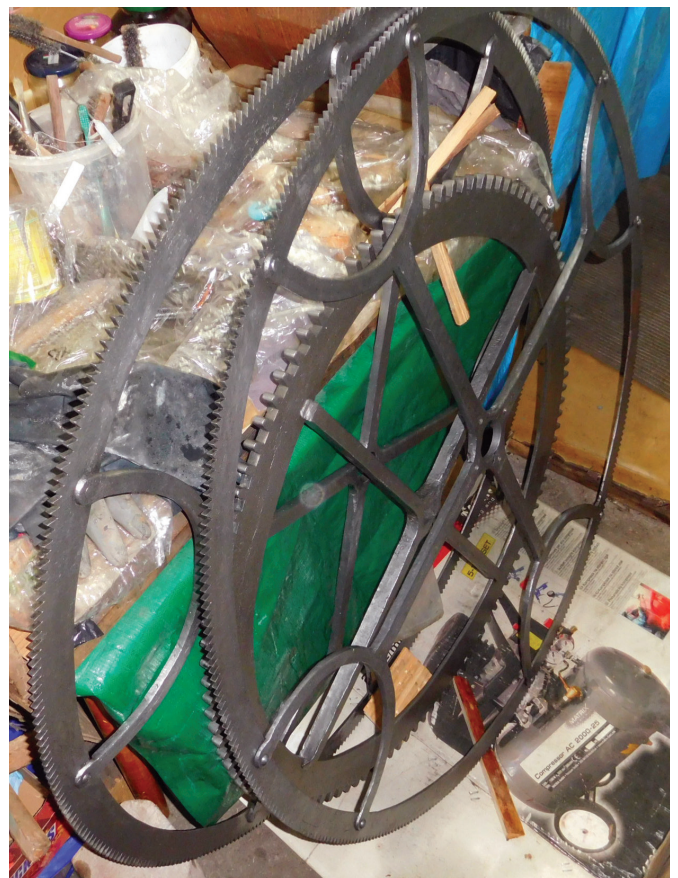
All the wheels of the astronomical dials are wrought iron.
