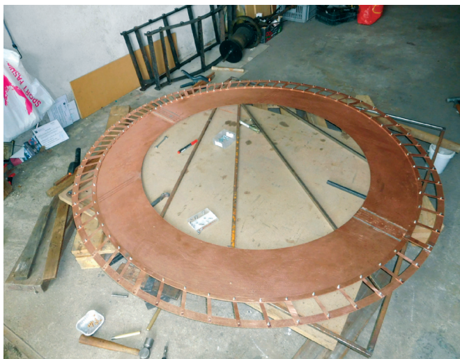
The original ecliptic ring with its zodiac figures was in poor condition. Petr has fabricated a new ring in copper. The steel screws will all be replaced with copper rivets.
