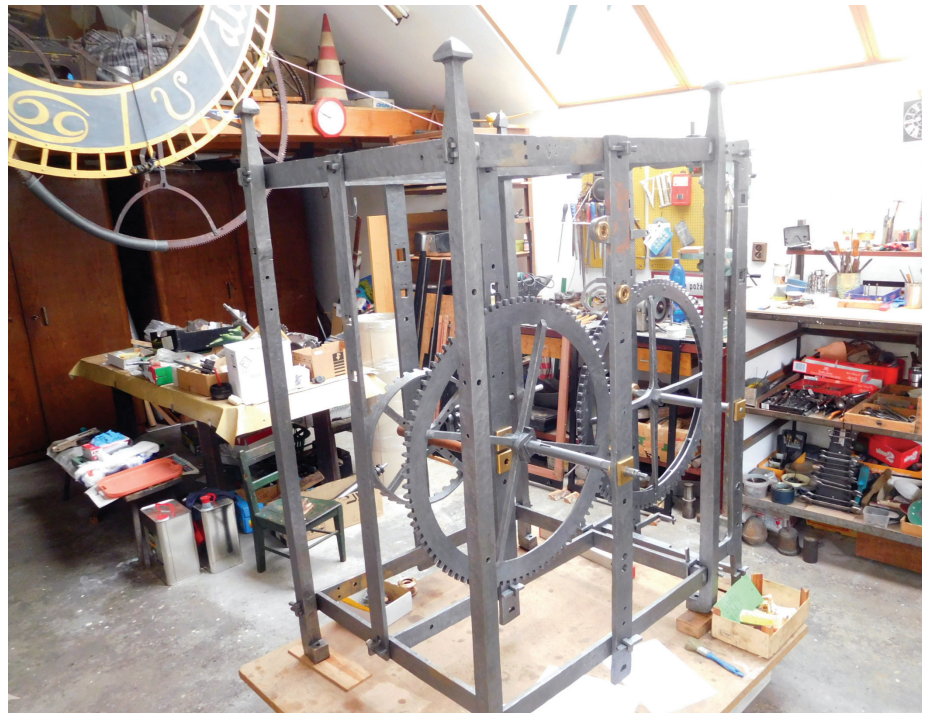
The going, striking and Apostles' carousel-drive, and all in one frame. Shown here is the basic frame; parts were later added.
