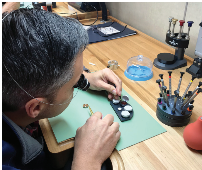
A student at the Build a Watch event lubricates the barrel arbor of his watch movement before installing it.
