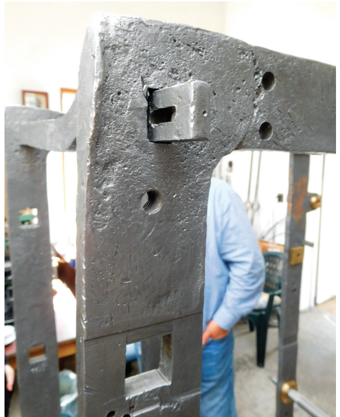
Cleaning has revealed how iron parts have been joined using welded scarf joints.
