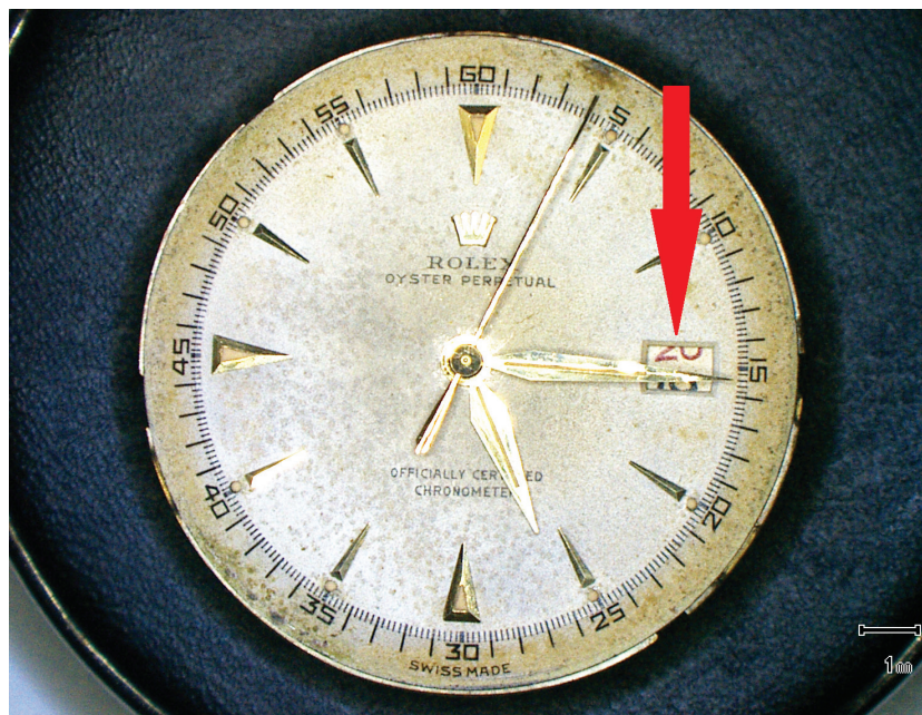
The date disc is stuck in the wrong position in relation to the date window.
