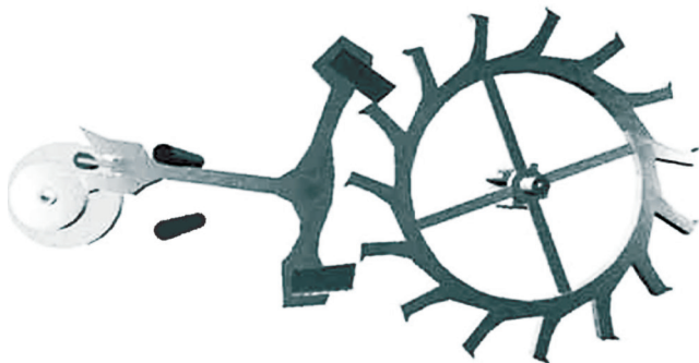
Figure 23. Unlocking of lever escapement.
