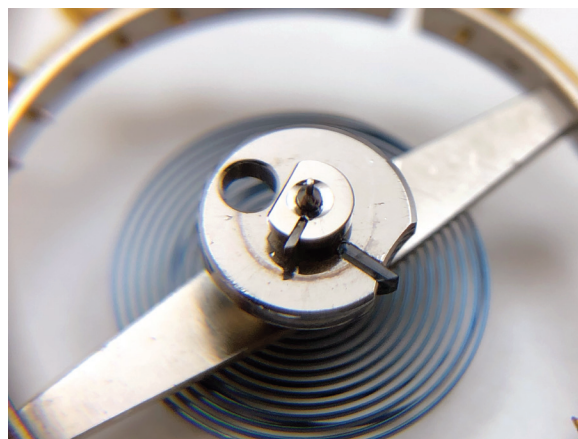
Fig. 8. Lower section of the balance wheel.
