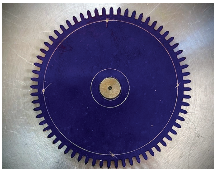
Fig. 4. The four strike marks with slight divots made at their intersections.
