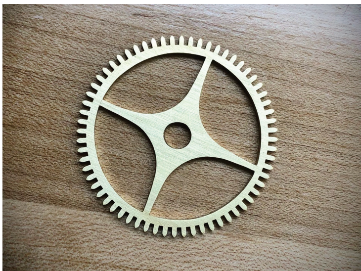
Fig. 7. The completed crossed wheel after piercing and filing.
