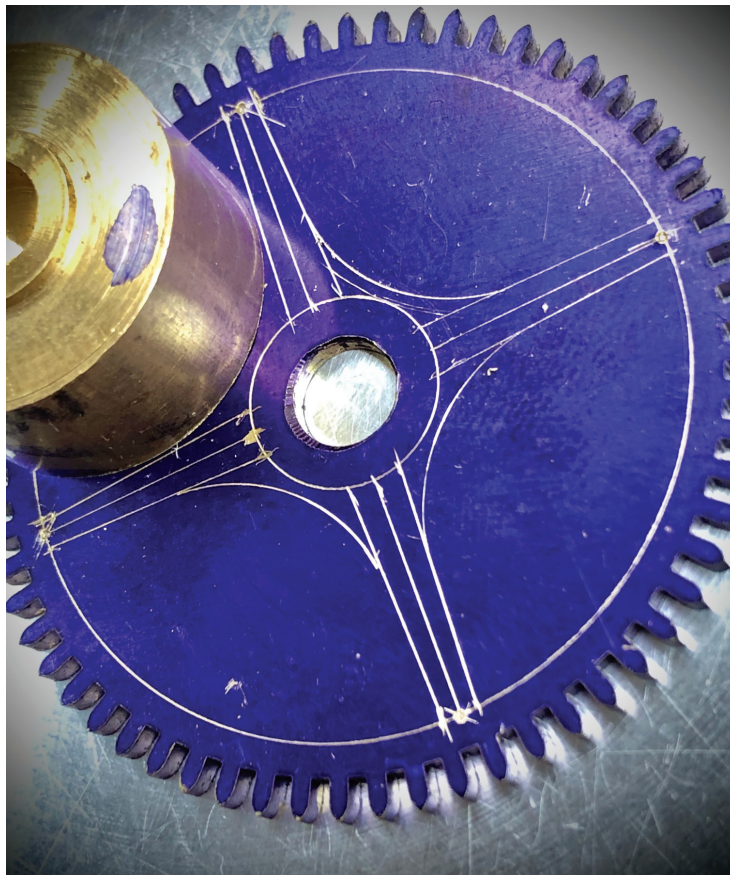
Fig. 6. Using a template to radius the spokes after tapers were drawn.
