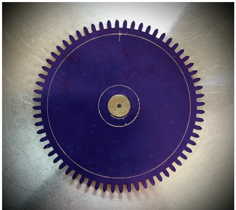
Fig. 2. Wheel with the upper- and lower-limit circles drawn and the starting mark in place.
