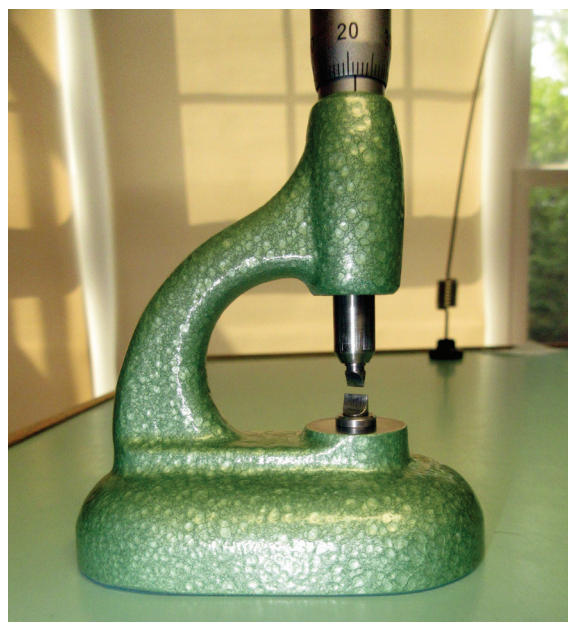
Fig. 3. Bergeon pusher and stump set, fitted to a Horia 4mm jewelry tool.
