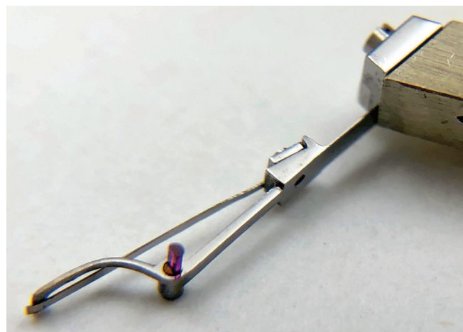
Fig. 6. Completed detent with locking jewel and passing spring.
