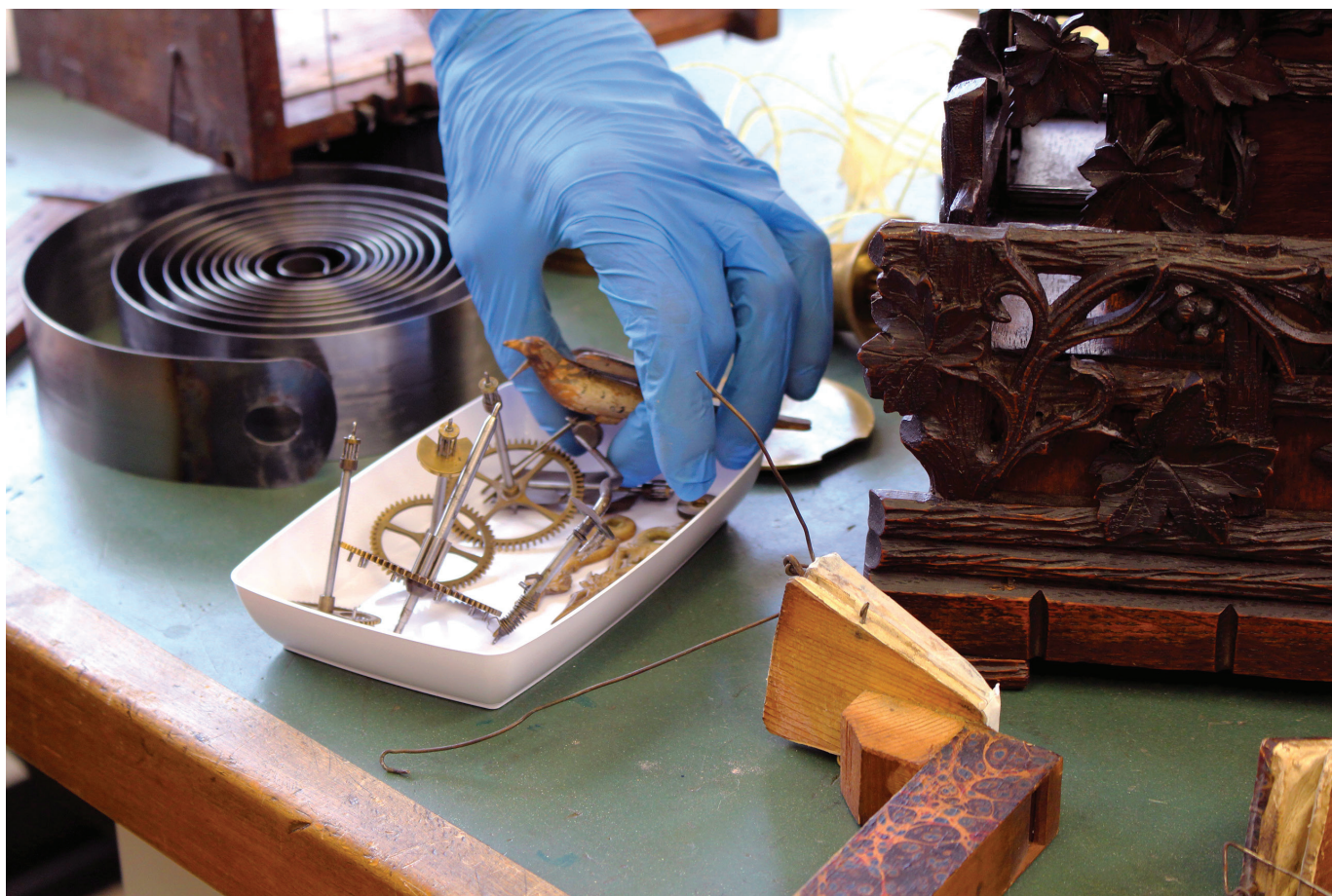
Fig. 2. The clock's pinions and cuckoo bird, during the restoration process.
