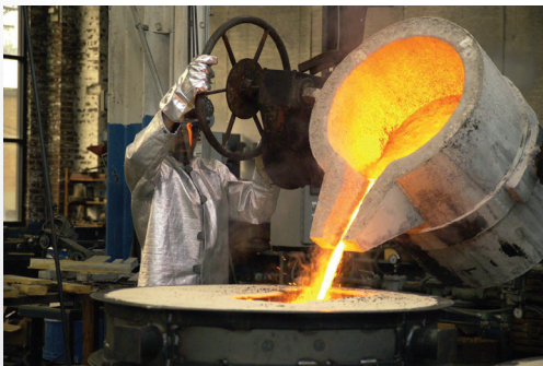
Pouring a bell at Verdin Bells & Clocks
