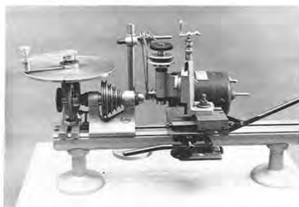
Figure 88. Dividing Head Mounted on Watchmaker's Lathe (Courtesy of Parkland College)
