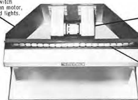
Inside View of Dust Collector
