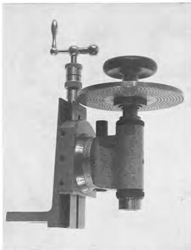
Figure 86. Milling Attachment Fitted with Index Plate (Courtesy of Parkland College)
