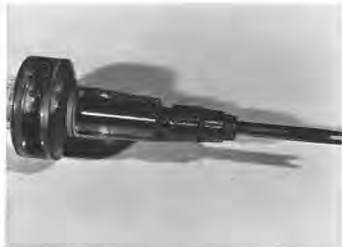
Figure 4. Liquid level screwdriver slotted to fit timing weights.
