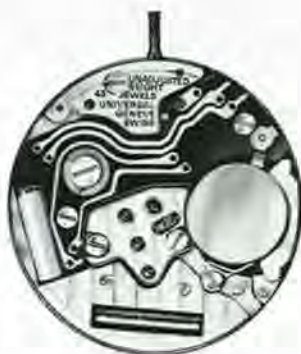
Caliber 43, Universal Geneve's new quartz movement demonstrating remarkable slimness (only 2.30 mm), is designed for use in both ladies' and men's extra-slim watches.
