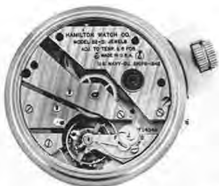
Figure 3. Hamilton 35 size Non-gimballed Chronometer Watch, Model 22. Same movement used in the Gimballed model. Note Safety Setting Push Pin in Case just to the Right of the Movement Number.
