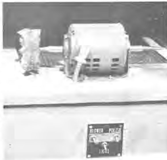
Figure 1. Polishing motor with two tapered spindles for quick change of buffs.
