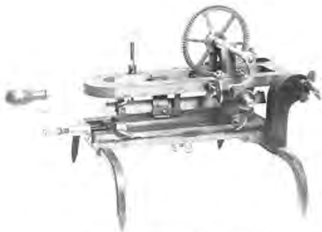
Chronometer Pinion Cutter from the William Bond & Son Shop. (Courtesy of the Smithsonian Institution)
