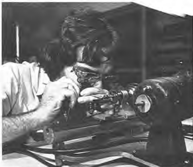
MATC horology student Michael Hannagan turns down a new pivot that has been set in a clock wheel arbor.
