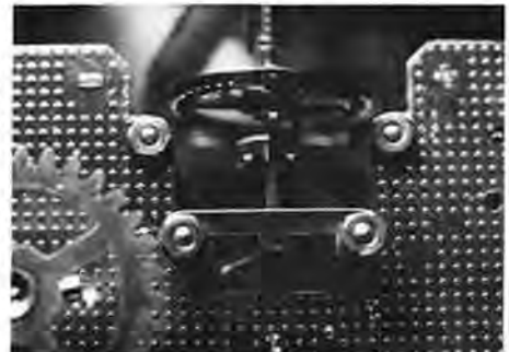
Figure 9. Drop has just occurred to the exit pallet. Note the position of the fork relative to the balance wire.
