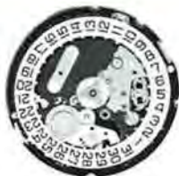
ESA 944.111 11½" Ø 25.60 mm. 3.10 mm thin. Center seconds. Date.
