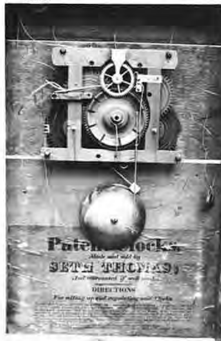
Figure 3. Terry 30-hour movement, strap model, number 2, before restoration; showing the label fastened to the backboard.
