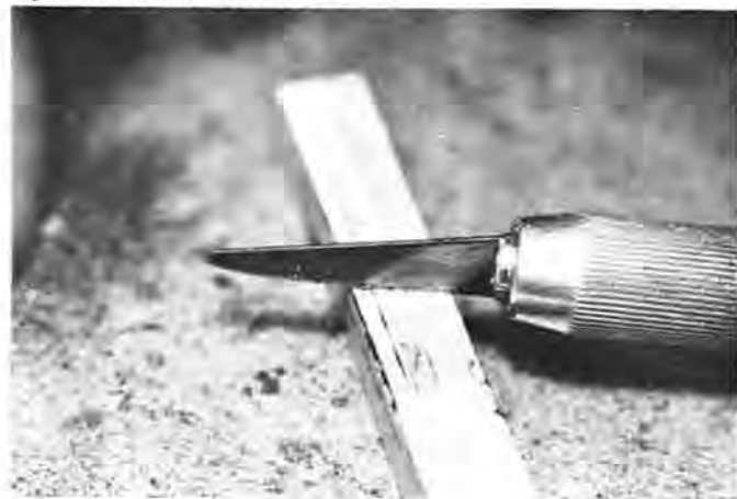
Figure 1. Scraping a boxwood lap true.
