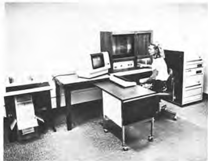
The Gemprint computer system includes a video digitizer and Digital Equipment computer that analyzes the diamond "fingerprints." Over $1 million worth of stolen diamonds have been identified by the Gemprint computer.
