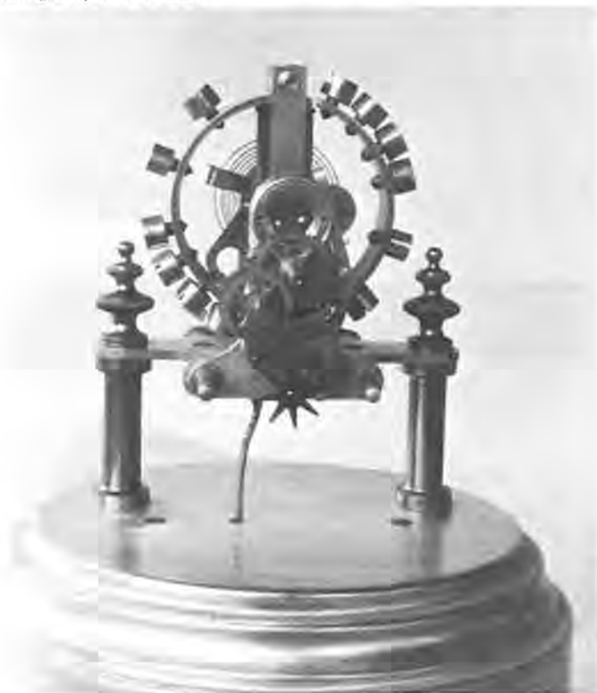
Figure 1. The rear of a "short" model Eureka, with a view of the rating star, dial removed.
