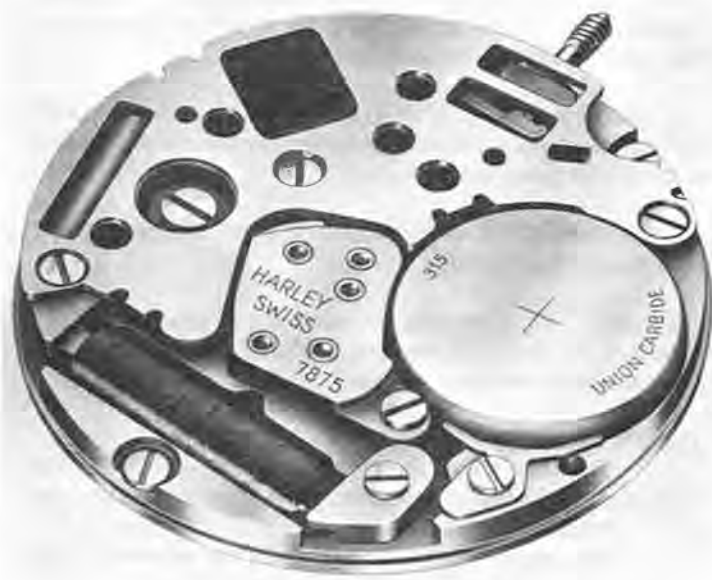
Only 1.95 mm thick, a new analog quartz movement designed for volume production at a highly competitive price. 8 1/4-line calibre (Ø 18.60 mm) with center seconds and date calendar. A 10 1/4-line version (Ø 23.30 mm) also 1.95 mm thick is planned (RONDA Harley Quartz 7873-7875).
