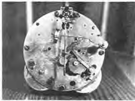
Figure 3. Rear of the movement, showing the rack and snail arrangement.
