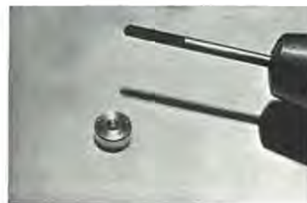
Figure 5. Bushing removed from drill, ready for finishing.
