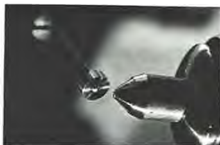
Figure 4. Hole drilled; bushing parted from rod.
