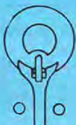
Figure 2. The Guard Pin passing through the crescent.
