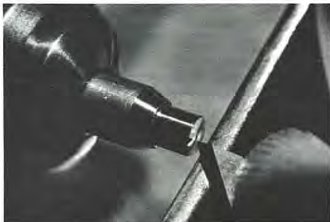
Figure 1. Brass rod turned to size, corner chamfered, and starting center cut.
