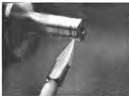
Figure 4. Making starting center for drilling pinning hole in collet. Bur is cutting radially into side of brass rod.
