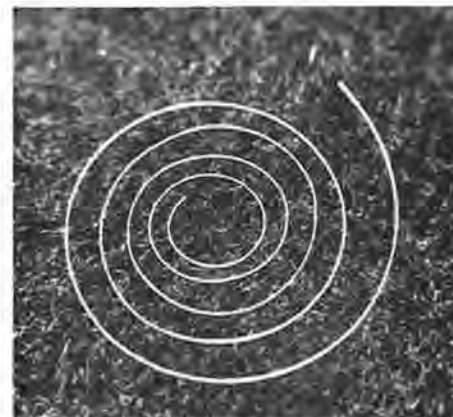
Figure 2. Hairspring trued and ready for colletting.
