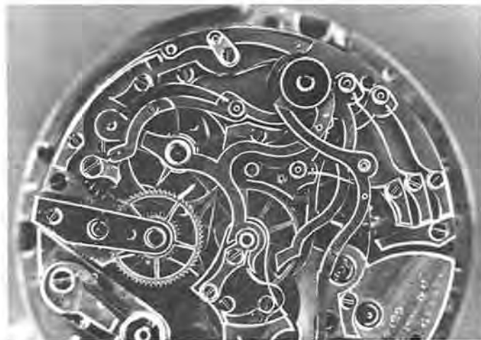
Figure 9. View of Stem Side of Upper Plate, showing some Chronograph levers and Wheels.
