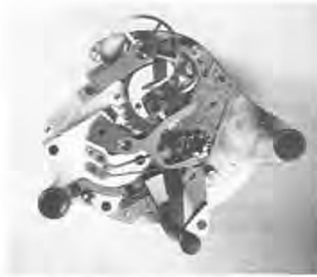
Figure 5. An under the dial or dial side of the pillar plate view of LeCoultre's second model. The large wheel at the 12 o'clock position is the time of flight hour wheel which carries the elapsed time hand.
