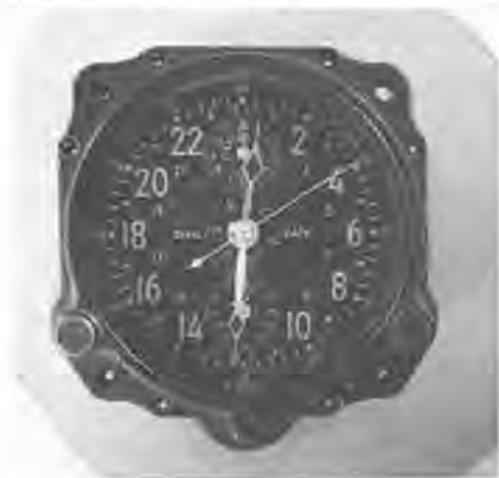
Figure 4. The dial of LeCoultre's second "Chronoflite" model.
