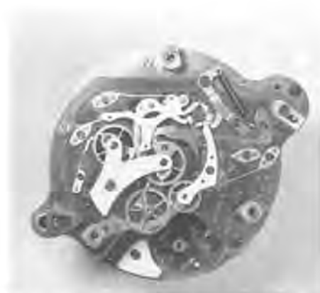
Figure 13. A view of the Elgin-Hamilton Elapsed Time Clock chronograph mechanism. This mechanism was responsible for starting, stopping and returning the sweep second and minute register hands to zero.
