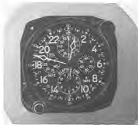
Figure 11. The dial of the Elgin-Hamilton 24-hour Elapsed Time Clock. The unmarked subsidiary dial at the 24-hour mark records each revolution of the sweep second hand up to 60 minutes, while the one at the 6 o'clock position is the continuous running second hand orbit.
