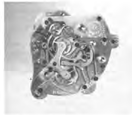
Figure 6. The chronograph mechanism which starts, stops, and returns the sweep second hand to zero.
