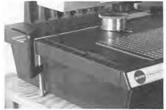
FIGURE 6. Straight-edge clamped to base of fiche reader to assist in realigning the work with the drawing.
