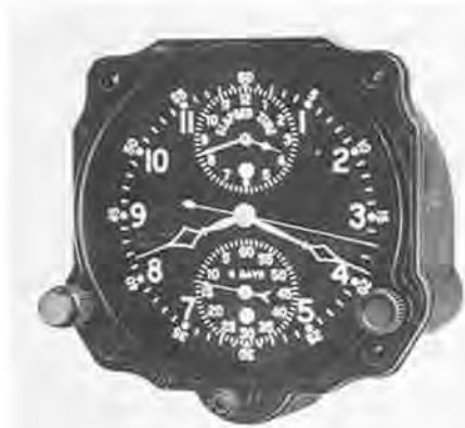
Figure 4. The dial of LeCoultre's second "Chronoflite" model.
