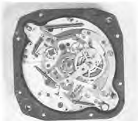
Figure 14. An under the dial view of elapsed time and civil date mechanism of the Elgin-Hamilton Elapsed Time Clock.
