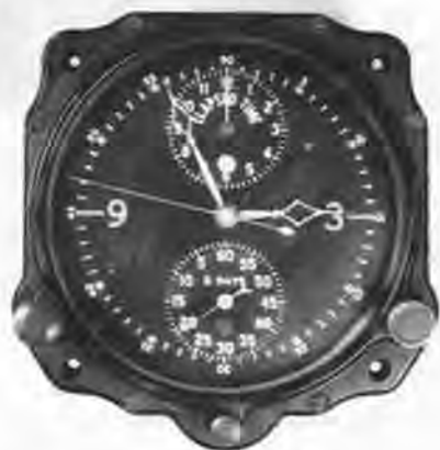
Figure 1. Dial view of LeCoultre's first "Chronoflite" Elapsed Time Clock.
