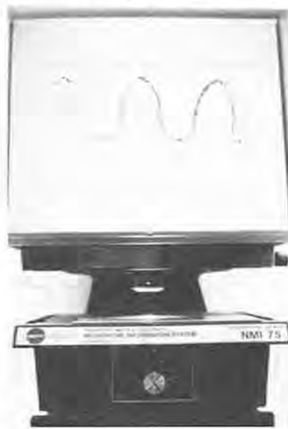
FIGURE 5. Tracing of clock wheel teeth (to assist in achieving proper spacing and profile when replacing broken teeth).
