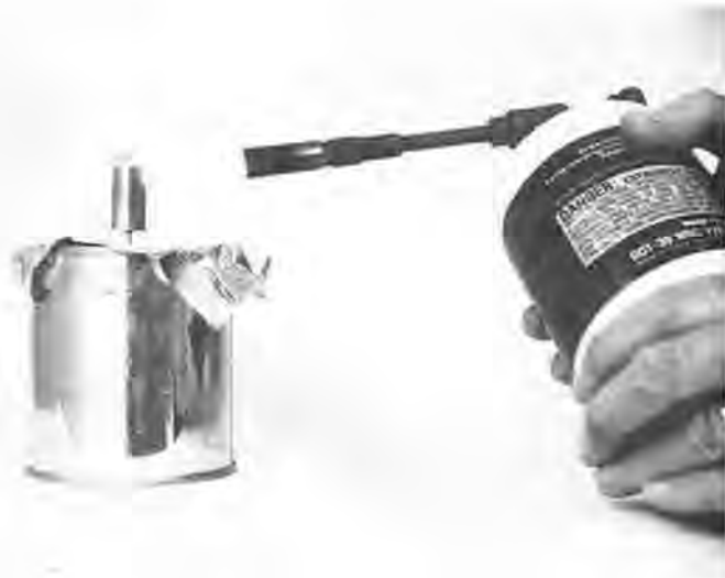
FIGURE 2. Flame is directed only to the brass heat sink.
