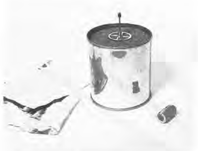
FIGURE 1. Example of center wheel-arbor-pinion, placed in secure position in can of clean sand, with sheets of aluminum foil at left, and brass slug heat sink at right.
