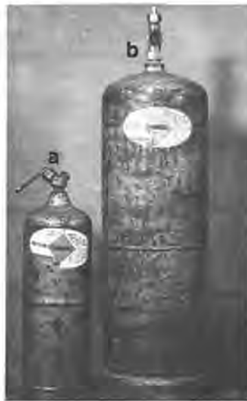
Figure 2a. "M.C." acetylene tank. Figure 2b. "B" acetylene tank.
