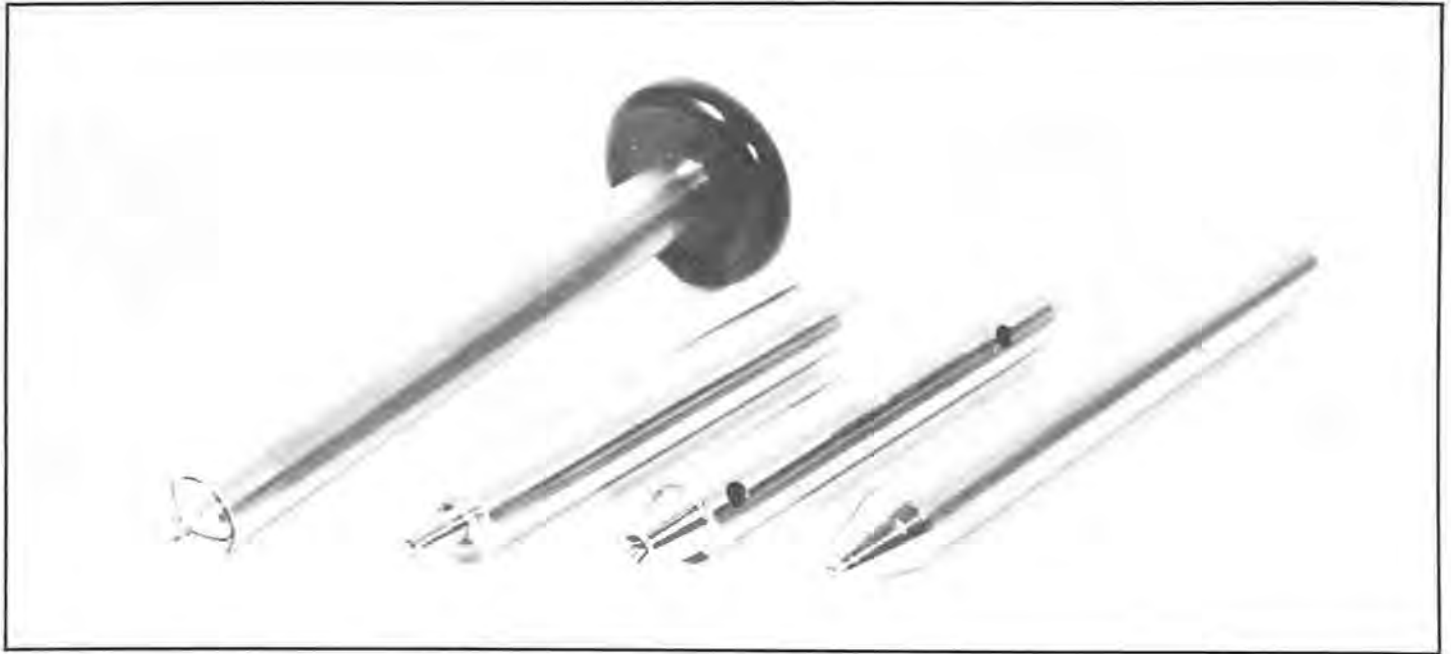
FIGURE 3. Chuck holding tailstock runner at left, typical female centering runners at right.
