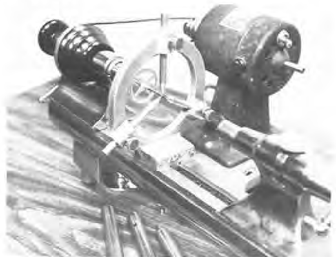
FIGURE 4B. Steady-rest runners are now evenly tightened down, and female runner in tailstock replaced by chuck-holding runner, preparatory to drilling.
