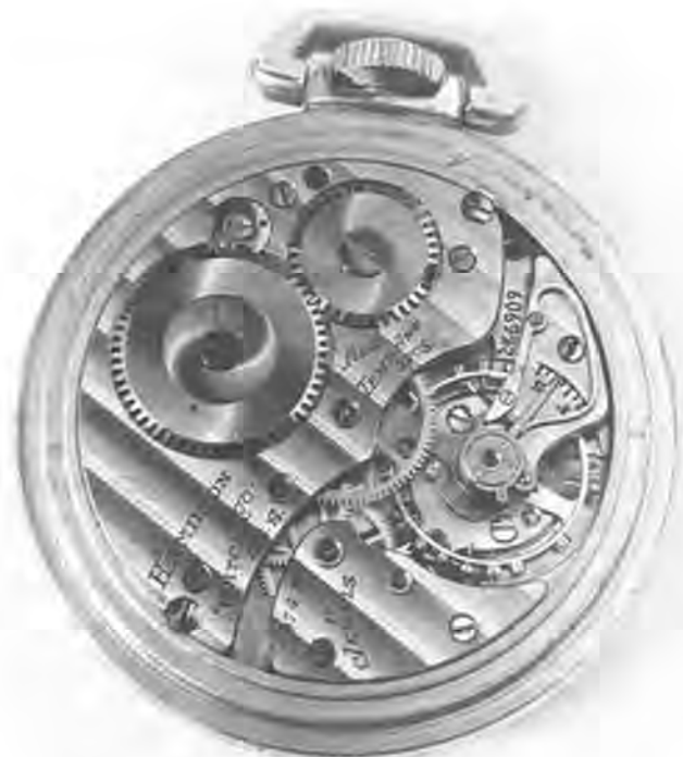
Figure 2. Movement view of Hamilton's model 2974B, 16 size, 17 jewels, Comparing Watch.
