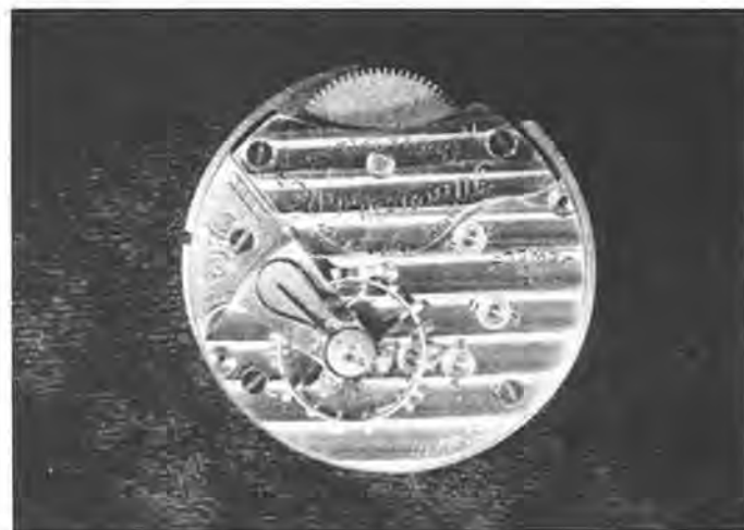
Figure 5. 18/s Illinois time lock movement removed from movement block.
