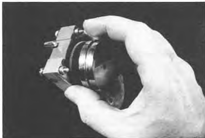
Figure 7. Removing barrelled mainspring/ratchet wheel assembly.
