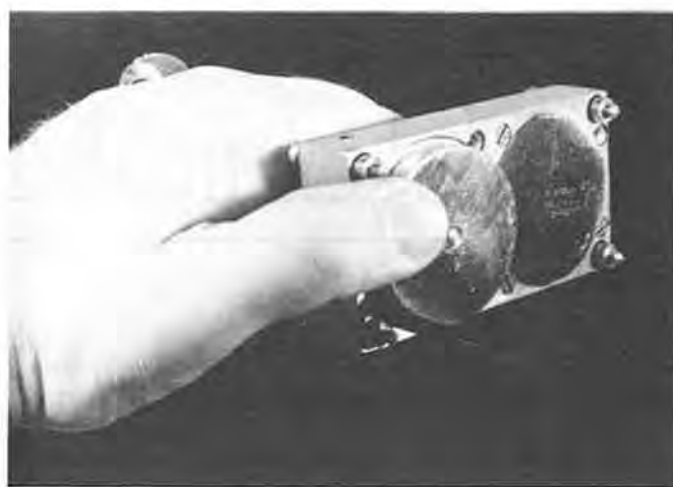
Figure 6. Releasing mainspring power (refer to text).
