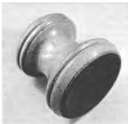
Hand-held screw back case opener.
