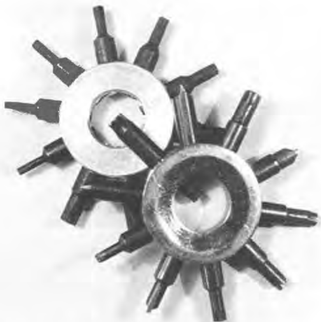
Figure 10. Two sleeve wrenches for removing and inserting sleeves.
