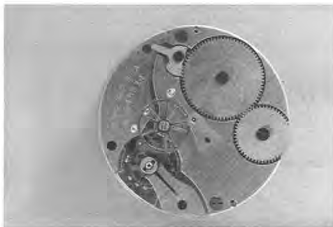
Figure 3 (top left). Movement view of Elgin's 22 size, 7 jewel, 8-day, Grade 562 Aircraft Clock. Note the spring loaded double sweep second wheel which prevents any backlash in the rotation of the sweep second hand.
