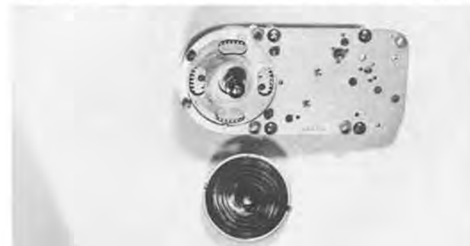
Figure 7. The "L"-type with barrel removed.
