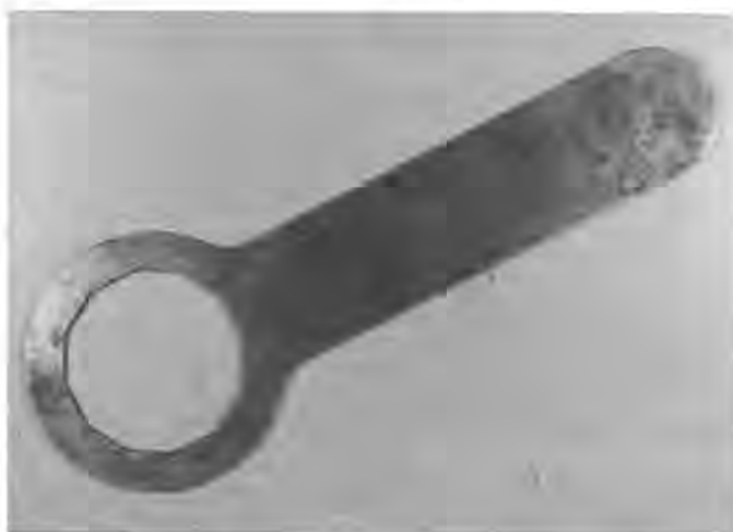
Figure 4 (right): Elgin dodecagon spanner wrench, 7¼ x 2½ inches, with 1¾-inch opening for opening and closing Elgin's 16-size waterproof timer.
