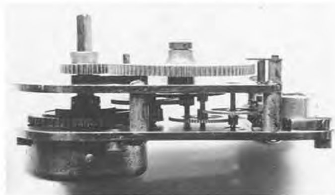
Figure 2. Side view of the Yale "L"-type movement showing 5-wheel train.
