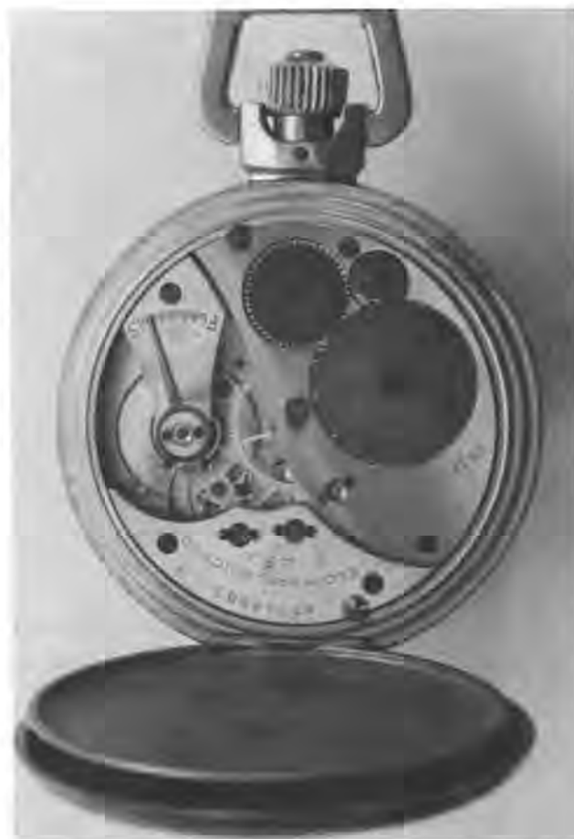
Figure 10. Elgin type A, 1/30-second timer, with very small balance wheel. A segment of the rim (light arc) is visible just to the right of the upper balance cock cup jewel. Movement No. 4181-9863, 16 size, 15 jewels.
