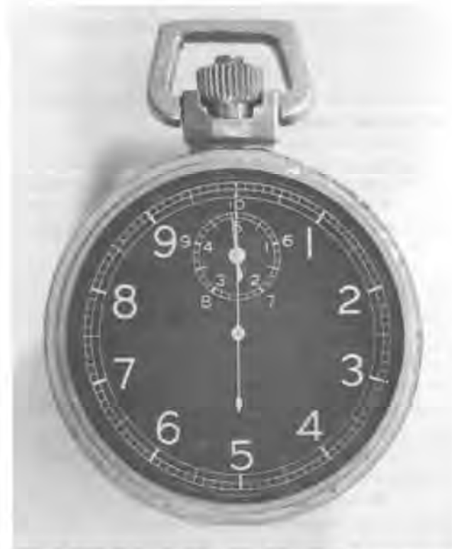
Figure 9. Elgin type A-8 1/30-second navigation (ground speed) timer. One revolution of the minute register hand, located under numeral "10" at 12 o'clock, equals 5 minutes. Movement No. 41819863, 16 size, 15 jewels.
