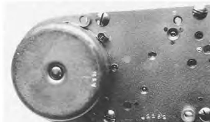
Figure 4. Lower plate of the "L"-type showing mainspring barrel. Note that the fourth and fifth wheels are jeweled.
