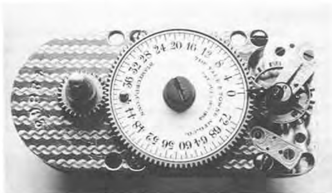
Figure 1. Yale "L"-type timelock movement.
