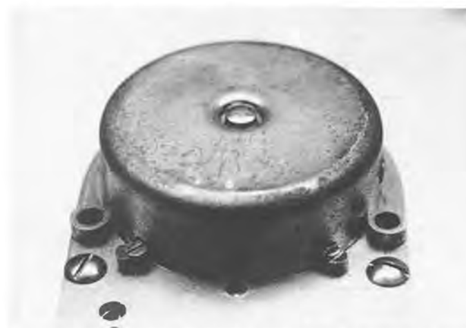
Figure 6. The mainspring barrel showing two barrel lug screws. The one on the right is in a locked position and the one on the left is unlocked.
