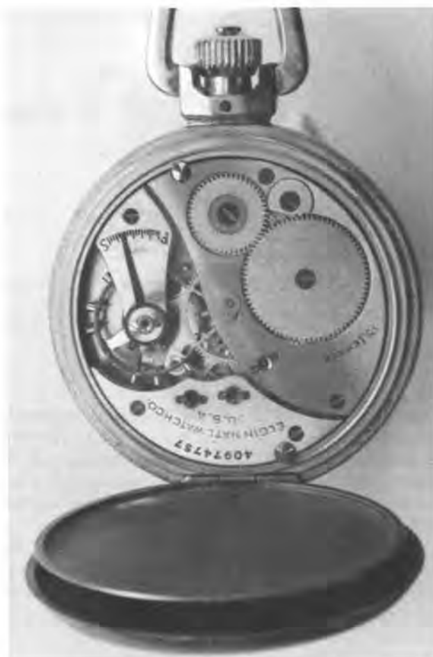
Figure 6. Elgin timer showing steel parts without black oxide finish. Movement number 40974757, 16 size, 15 jewels.
