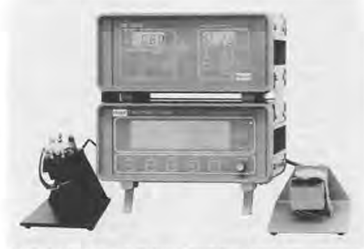
Vibrograf's Timoquartz 4500 Quartz Watch Rate Timer shown mounted on Timoprint 4500 Mechanical Watch and Rate Recorder.
