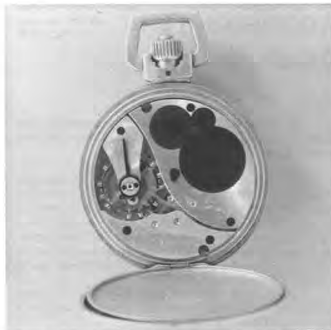
Figure 7. Elgin timer showing steel parts with black oxide finish to prevent corrosion. Movement number 41816068, 16 size, 15 jewels.
