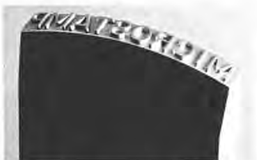
Figure 2. Enlarged micro-stamp tip shows how "roll on" design allows each letter to get full, clean impression.
